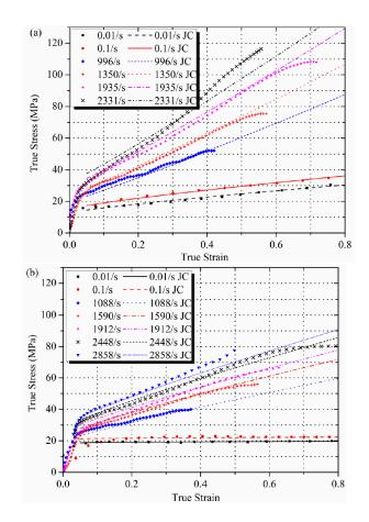
**Figure 8.** Comparison of Johnson-Cook model to (**a**) low crystalline and (**b**) high crystalline Al-PTFE experimental data.
