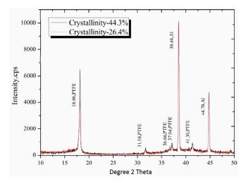
Figure 3. X-ray diffraction patterns of low and high crystalline Al-PTFE.
