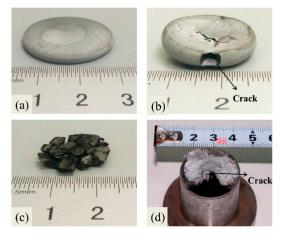
**Figure 9.** Recovered Al-PTFE samples after compression. (**a**) High crystalline sample after quasi-static compression; (**b**) Low crystalline sample after quasi-static compression; (**c**) Low crystalline sample after SHPB tests; (**d**) High crystalline sample after drop weight tests.
