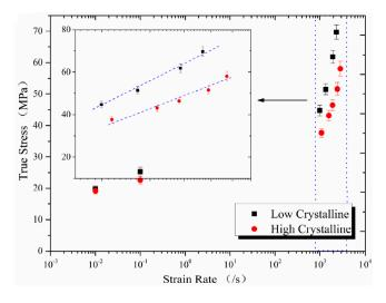
**Figure 7.** Comparison of true stress as a function of log (strain rate) between low crystalline and high crystalline Al-PTFE.
