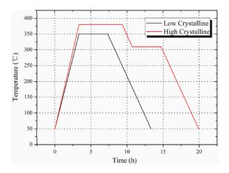
Figure 1. The sintering procedure of low and high crystalline Al-PTFE samples.
