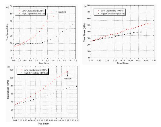
**Figure 6.** Comparison of stress-strain curves between low crystalline and high crystalline Al-PTFE at (a) strain rate of 0.01 s<sup>-1</sup>; (b) strain rate of about 1000 s<sup>-1</sup>; and (c) strain rate of about 2300 s<sup>-1</sup>. The point where the reaction took place is marked.
