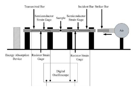
Figure 2. Schematic illustration of the SHPB system.
