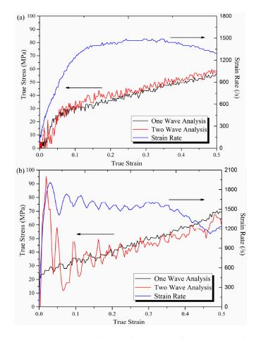
**Figure 5.** One-wave versus two-wave analysis and strain rate of Al-PTFE (**a**) with pulse shaping and (**b**) without pulse shaping.
