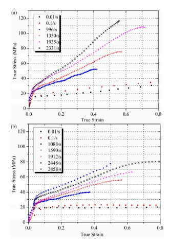
**Figure 4.** Stress-strain curves of (**a**) low crystalline and (**b**) high crystalline Al-PTFE tested in compression at room temperature.
