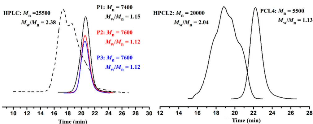
**Figure 3.** The GPC curves of the linear poly( $\epsilon$ -caprolactone) (P1,  $M_n$  GPC = 7400 g/mol,  $M_w/M_n$  = 1.15; PCL4,  $M_n$  GPC = 5500 g/mol,  $M_w/M_n$  = 1.13), hyperbranched poly( $\epsilon$ -caprolactone) (HPCL,  $M_n$  GPC = 25,500 g/mol,  $M_w/M_n$  = 2.38; HPCL2,  $M_n$  GPC = 20000 g/mol,  $M_w/M_n$  = 2.04).
