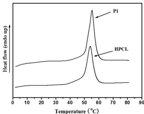
**Figure 7.** Second DSC heating curves of the linear poly( $\epsilon$ -caprolactone) (P1,  $M_{n\text{ GPC}} = 7400$  g/mol,  $M_w/M_n = 1.15$ ) and hyperbranched poly( $\epsilon$ -caprolactone) (HPCL,  $M_{n\text{ GPC}} = 25,500$  g/mol,  $M_w/M_n = 2.38$ ).
