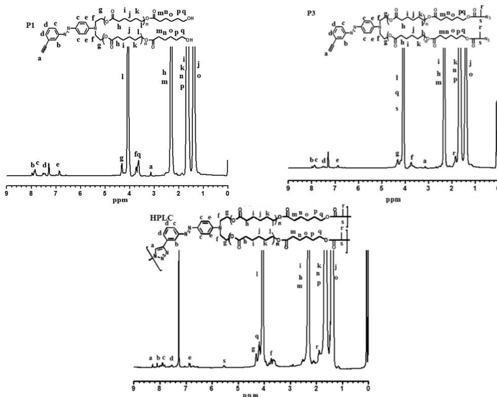
**Figure 4.**  $^1\text{H}$  NMR spectra of the linear poly( $\epsilon$ -caprolactone) (P1,  $M_n$  GPC = 7400 g/mol,  $M_w/M_n$  = 1.15), AB<sub>2</sub> macromonomer (P3) containing terminal ethyne and azide groups and hyperbranched poly( $\epsilon$ -caprolactone) (HPCL,  $M_n$  GPC = 25,500 g/mol,  $M_w/M_n$  = 2.38).
