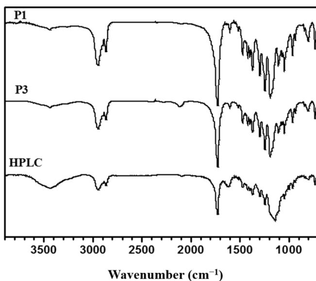
**Figure 6.** FT-IR spectra of the linear poly( $\epsilon$ -caprolactone) (P1,  $M_n$  GPC = 7400 g/mol,  $M_w/M_n$  = 1.15), AB<sub>2</sub> macromonomer (P3) containing terminal ethyne and azide groups and hyperbranched poly( $\epsilon$ -caprolactone) (HPCL,  $M_n$  GPC = 25,500 g/mol,  $M_w/M_n$  = 2.38).
