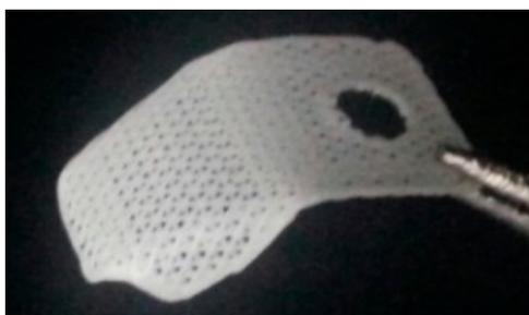
**Figure 5.** A PCL/PLGA/ $\beta$ -TCP membrane produced using 3D printing technology. Pores were triangularly structured and completely interconnected.
