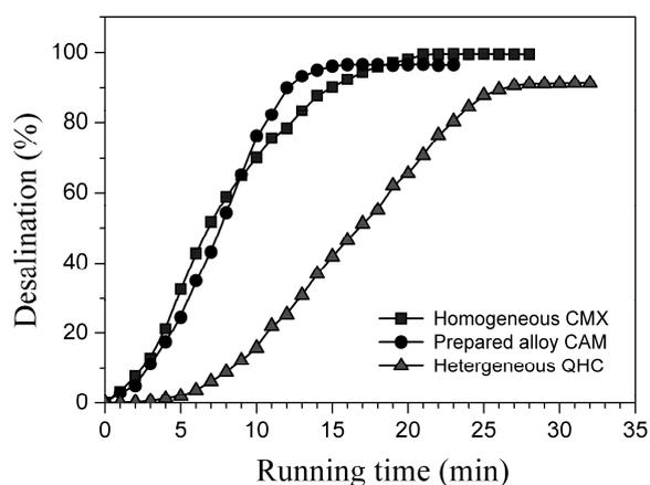
**Table 3.** Desalination effects of the cation exchange membranes <sup>a</sup>.
