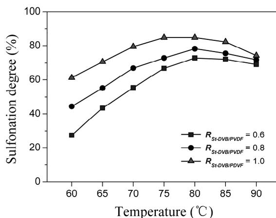
Figures 5 and 6 demonstrate the effects of PVDF content (represented by  $R_{St-DVB/PVDF}$ ) and DVB content in the polystyrene/PVDF alloy particles on the sulfonation degree, respectively. As shown in Figure 5, both the sulfonation degree and the experimental ion exchange capacity ( $IEC_{Experiment}$ )
