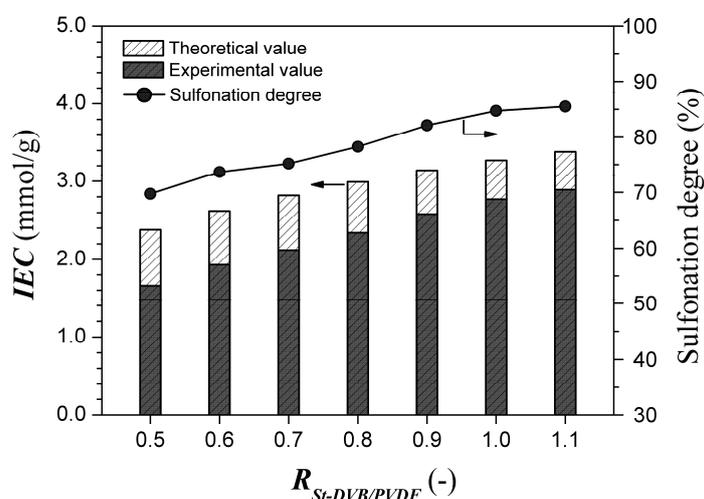
**Figure 6.** Ion exchange capacities and sulfonation degrees at various DVB contents. One hundred grams of polystyrene/PVDF alloy particles ( $R_{\text{st-DVB/PVDF}} = 0.8$ ) were reacted with 100 mL of DCE and 600 mL of concentrated sulfuric acid at 80 °C for 8 h.
