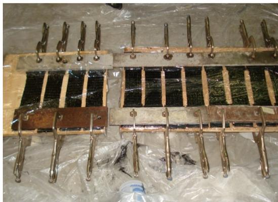
**Figure 3.** CFRP Coupon.
