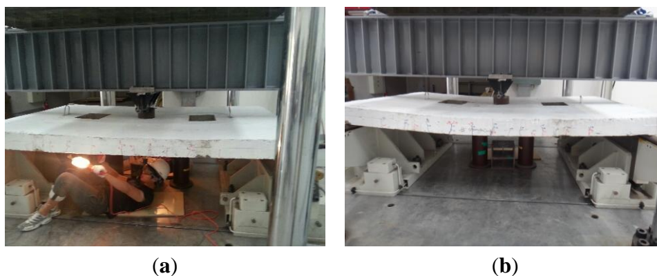
Figure 4. Test setups of (a) unstrengthening; (b) surround strengthening; (c) diagonal strengthening; (d) parallel strengthening for the various strengthening configuration.
