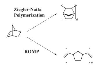
The development of ROMP is also documented in the academic literature [125–128]. The driving force for ROMP is the release of the ring strain enthalpy and, since the number of molecules is considerably reduced by polymerization, a positive ( $-T\Delta S$ ) must be compensated by the enthalpy term in order for the reaction to proceed according to:
