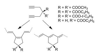
**Figure 58.** The ring-closure metathesis polymerization of  $\alpha$ ,  $\omega$ -dialkynes.
