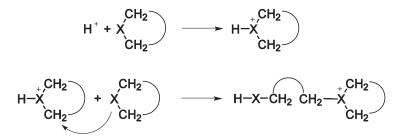
Alternatively, the heteroatom poly-acids of the general structure shown in Figure 17 can be employed as initiators [47].
