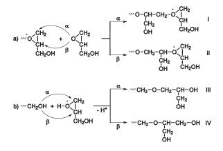
The experimental results suggest that the predominant structure is III [38,79,80] (Figure 31) so that it can be assumed that for this monomer the activated monomer mechanism predominates.
