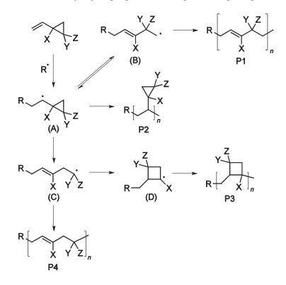
Which of the simple ROP products P1 and P4 predominates depends on the substituents Y and Z and the preference of the ring to open at the  $CX-CH_2$  or the CX-CY bond. The simple vinyl chain polymerization P2 and the intermediate formation of a four-membered ring to yield P3 are additional possibilities.
