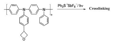
If the hole defect polymer has numerous oxetane side groups, the ROP leads to crosslinking and the polymer becomes insoluble. The soluble polymer can be coated (e.g., by spin-coating), dried and then photochemically crosslinked so that further coating is possible without dissolving the deposited film [71,72].
