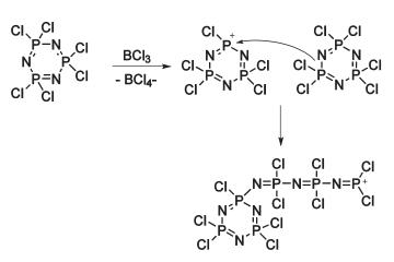
Figure 65. The cationic polymerization of hexachloro cyclo-triphosphazene.
