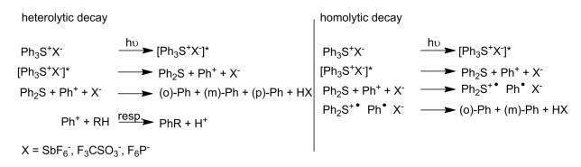
Via the heterolytic splitting of the initiator can be considered as an acid generator or photoacid generator (PAG). Typical examples are triphenylsulfonium triflate and diphenyliodonium triflate. The latter has been studied recently [66] to selectively cleave the carbon-oxygen bonds in a vinyl functionalized oxasilaspirocycle to form both homo- and copolymer polysiloxanes via a double ring-opening CROP (*cf.* Section 2.3, see Figure 23).
