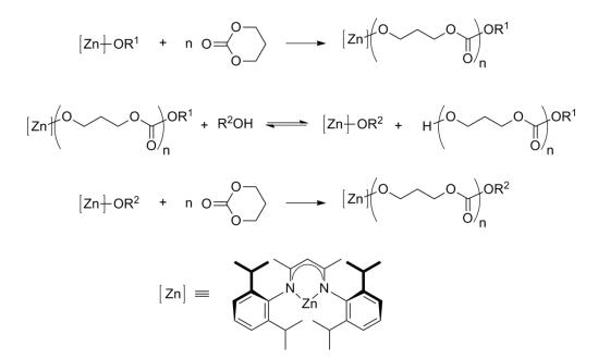
The initiators based on porphyrin complexes or complexes with related structures based on Al, Zn, Y, Lu, In have been used for the polymerization of e.g., oxiranes, thiiranes, lactones, lactides, cyclic
