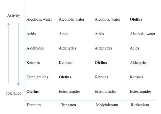
Figure 56. The reactivity/tolerance of metathesis catalysts.
