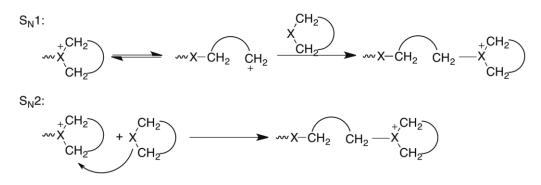
The polymer structure can be further controlled by the use of appropriate side groups. Thus, the exchange of an ether side group for an ester or carbamate (So-called NGP: Neighboring Group Participation) results in a different, well defined, microstructure during the CROP of cyclic dithiocarbonates (Figure 12) with methyl triflate initiator due to effective suppression of the isomerization of the monomer and the stabilization of the growing chain via the ester (carbamate) moiety [40].
