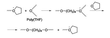
Since these reactions usually only become predominant when the monomer becomes depleted, only then do they represent chain termination rather than transfer; the charged species cease to grow due to lack of monomer and the second stage of the scheme in Figure 34 does not occur.
