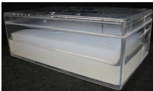
Silica gels were first mentioned in 1640 [1] and remained a curiosity until their adsorption properties were found to be useful. Dried silica gel is used, for example, as a desiccant because of its highly hygroscopic properties. The manufacturing is carried out by mixing water glass ( $\text{Na}_2\text{SiO}_3 \cdot x\text{H}_2\text{O}$ ) with acid. This work pursues the goal to quantify the consolidation of silica gels and gel fragments.
