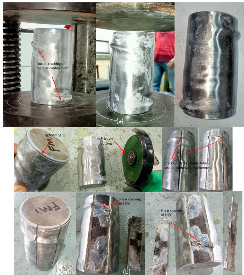
**Figure 12.** Failure modes of TSPC with fully metal tube confinement. (a) FM sample condition after mechanical testing. (b) The cut open of metal tube confinement for internal failure examination.
