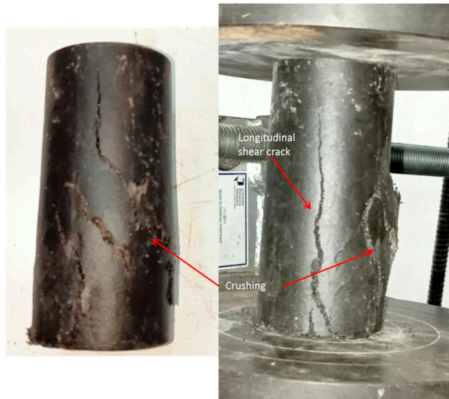
**Figure 10.** Failure modes of unconfined TSPC (UC).
