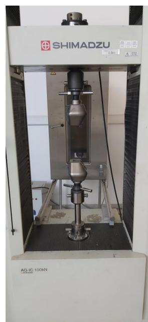
**Figure 8.** SHIMADZU Universal Testing Machine [21].
