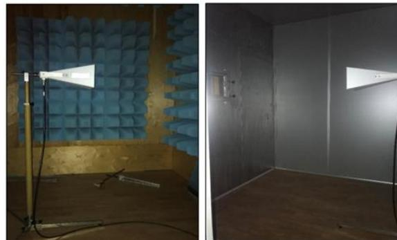
**Figure 6.** Shielded rooms with transmitting and receiving antennas [21].
