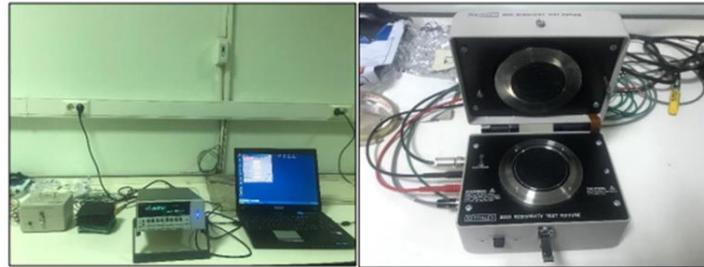
**Figure 7.** Pictures of an electrical resistivity test fixture [21].
