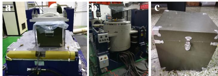
**Figure 2.** Vibration resistance testing of consolidated soil columns. (a) LS437A/BT900M(4T) Vibration Table; (b) MPA3324/H1248A (10T) vibration table; (c) Sample box.
