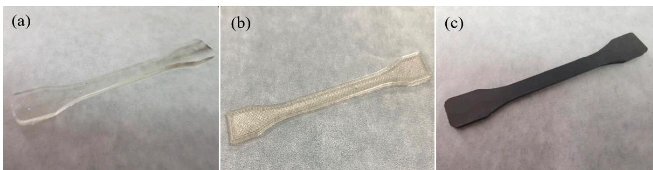
**Figure 2.** The tensile samples of (a) the injected PLA sample; (b,c) 3D-printed PLA and CNT/PLA samples.
