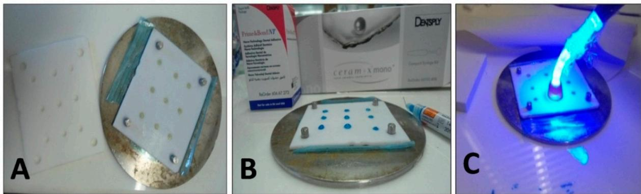
**Figure 1.** (A–C): Pictorial description of specimen's fabrication. (A) Mold filled with base material in first sheet. (B) Phosphoric acid gel applied on base material. (C) Composite filled in second sheet of Teflon sheet, added on top of the first sheet and material cured with LED light.
