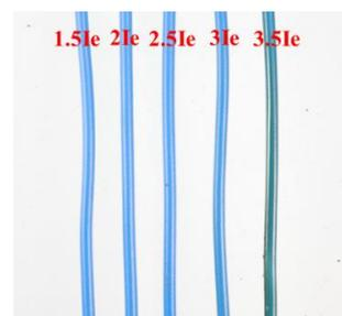
**Figure 2.** Various overload current PVC copper wires.
