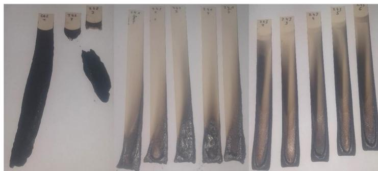
**Figure 1.** Burnt specimens after UL-94 V testing (1.6 mm). From left to right: PA\_1 to PA\_3.
