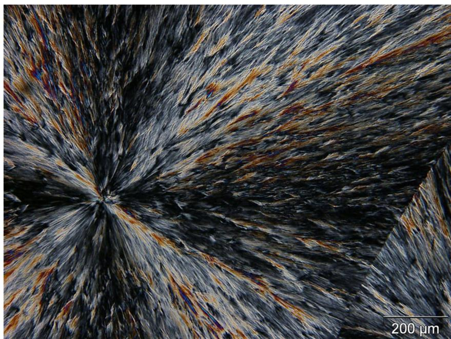
**Figure 3.** PEG spherulites observed by optical microscopy in combination with polarized light at ambient temperature.
