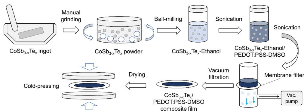
**Scheme 1.** Schematic diagram of the preparation of the  $\text{CoSb}_{3-x}\text{Te}_x$  skutterudite/PEDOT:PSS film.
