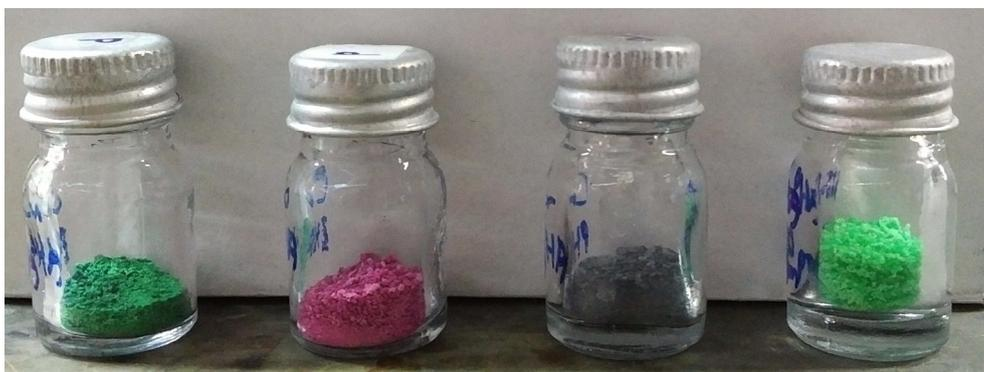
**Figure 1.** Poly(hydroxamic acid) with metal complex as the ligand-Cu (left), ligand-Co (second left), ligand-Cr (third from left), and ligand-Ni (utmost right).
