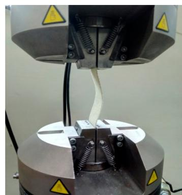
**Figure 7.** Buckling of a composite sample.
