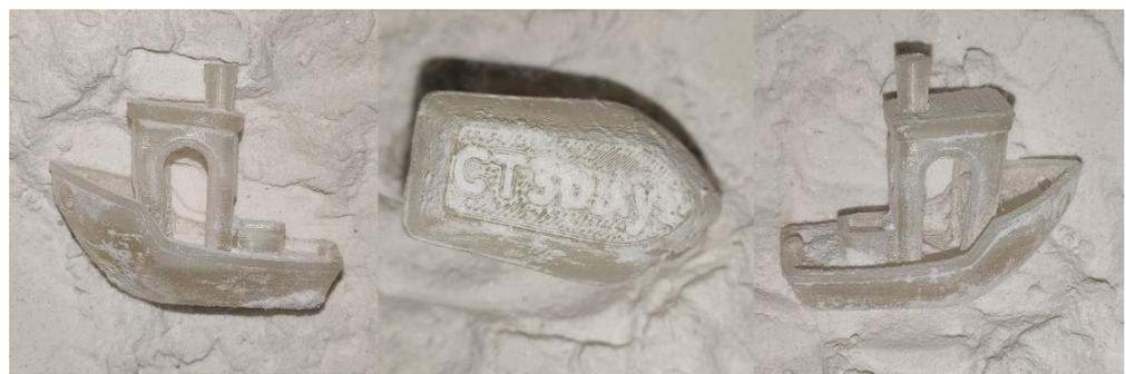
**Figure 15.** Images of a 3DBenchy (all instances shown are after heat treatment).
