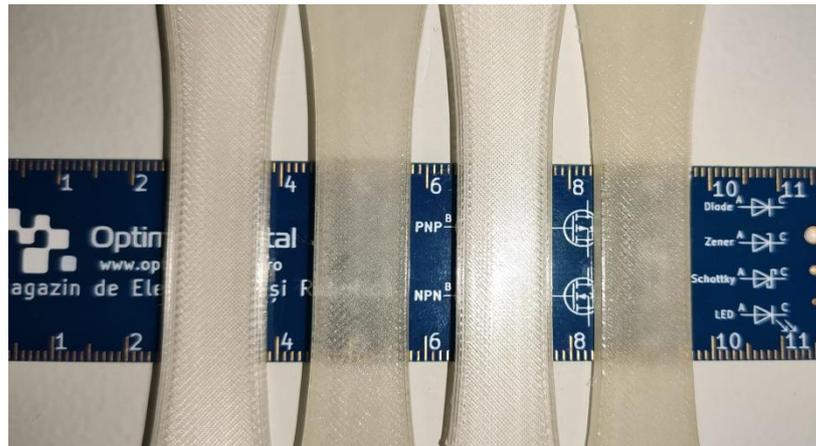
**Figure 16.** Visual changes observed in optical properties after heat treatment of horizontal orientation 3D printed parts. Lighter parts are untreated samples from the control group and darker parts are samples after full heat treatment. No other processing was done to the samples.
