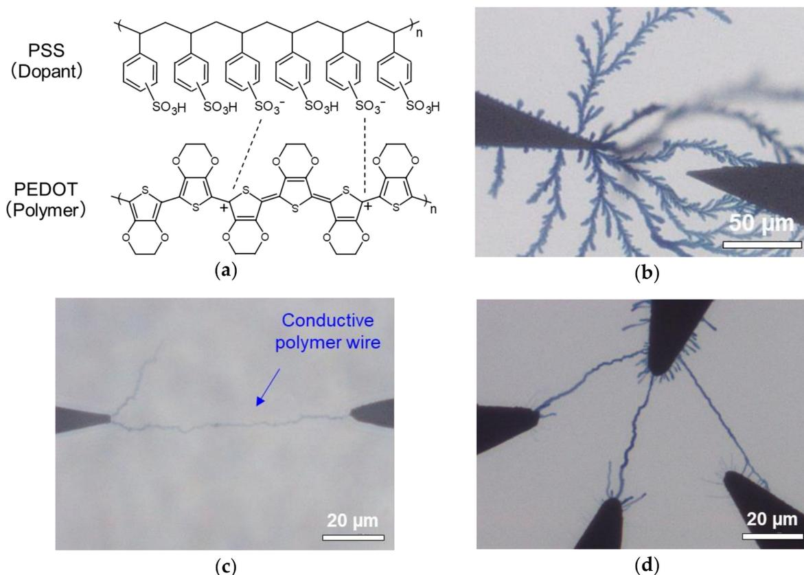
**Figure 1.** (a) Molecular structure of poly(3,4-ethylenedioxy-thiophene) doped with poly(styrene sulfonate) anions (PEDOT:PSS) conductive polymer. (b) Dendritic and (c) wire-shaped PEDOT:PSS obtained via electrodeposition. (d) Network circuit formed via branch wiring of PEDOT:PSS polymer between four electrodes.
