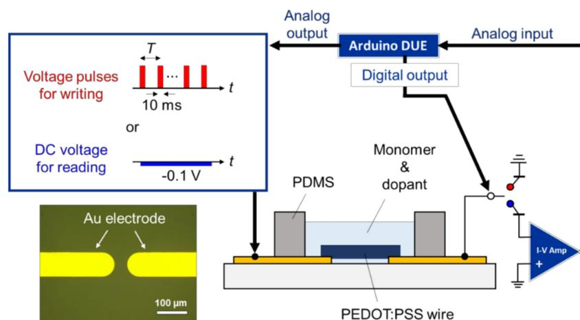
**Figure 2.** Schematic diagram of the experimental setup with a corresponding optical microscope image of the Au electrode gap. During conductance writing, the microcomputer supplied continuous voltage pulses and the counter electrode was switched to ground (GND). During conductance reading, the microcomputer supplied a  $-0.1$  V DC voltage and the counter electrode was switched to the I-V amplifier.
