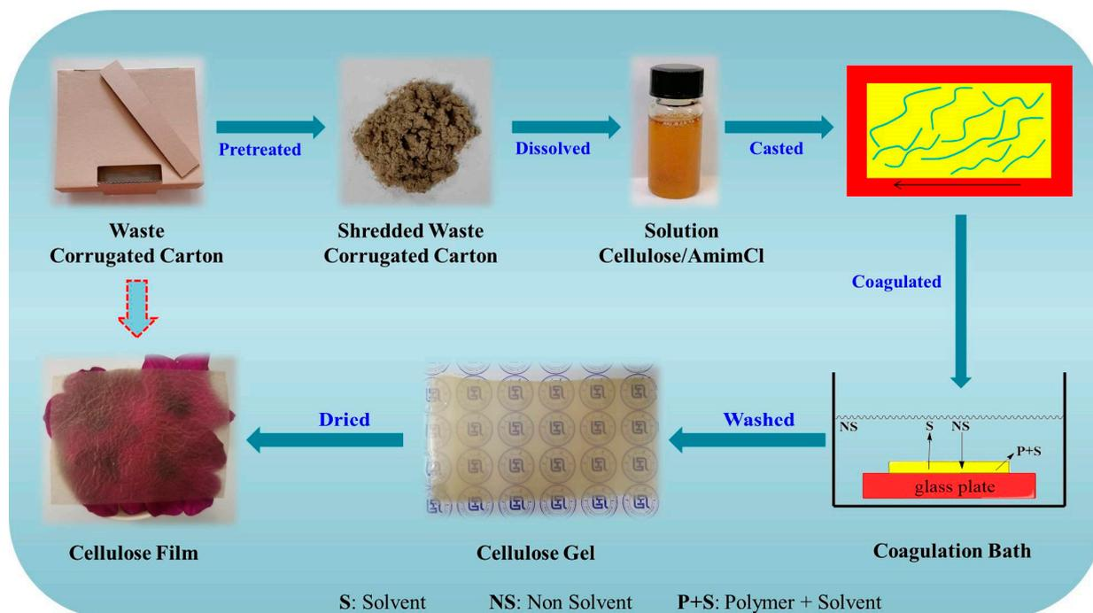
**Figure 1.** Preparation scheme of cellulose-based films from old waste corrugated cartons.
