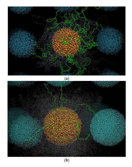
**Figure 9.** Typical atomistic snapshots of the nanoparticle network formed in: (a) the  $d5_v15_PEG$ , and (b) the  $d9_v15_PEG$  nanocomposite (T = 413 K and p = 1 atm). With yellow, red, and white we show the silica atoms. With blue we indicate images of the silica nanoparticle in neighboring cells. Non-bridging chains are shown in red, white, and cyan, and bridging ones in green.
