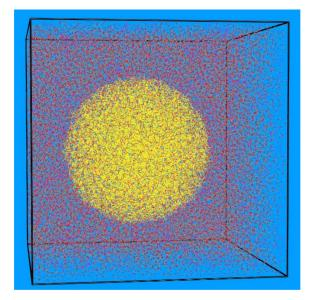
**Figure 1.** Typical atomistic configuration in box-relative coordinates of the d9\_v15\_PEG system (system 4 in Table 1) containing 750 PEG chains with degree of polymerization N = 41 and one spherical silica nanoparticle of diameter d = 9 nm in a cubic simulation cell with dimensions equal to 138 Å × 138 Å. Carbon, oxygen, hydrogen and silica atoms are shown with gray, red, white, and yellow color, respectively.
