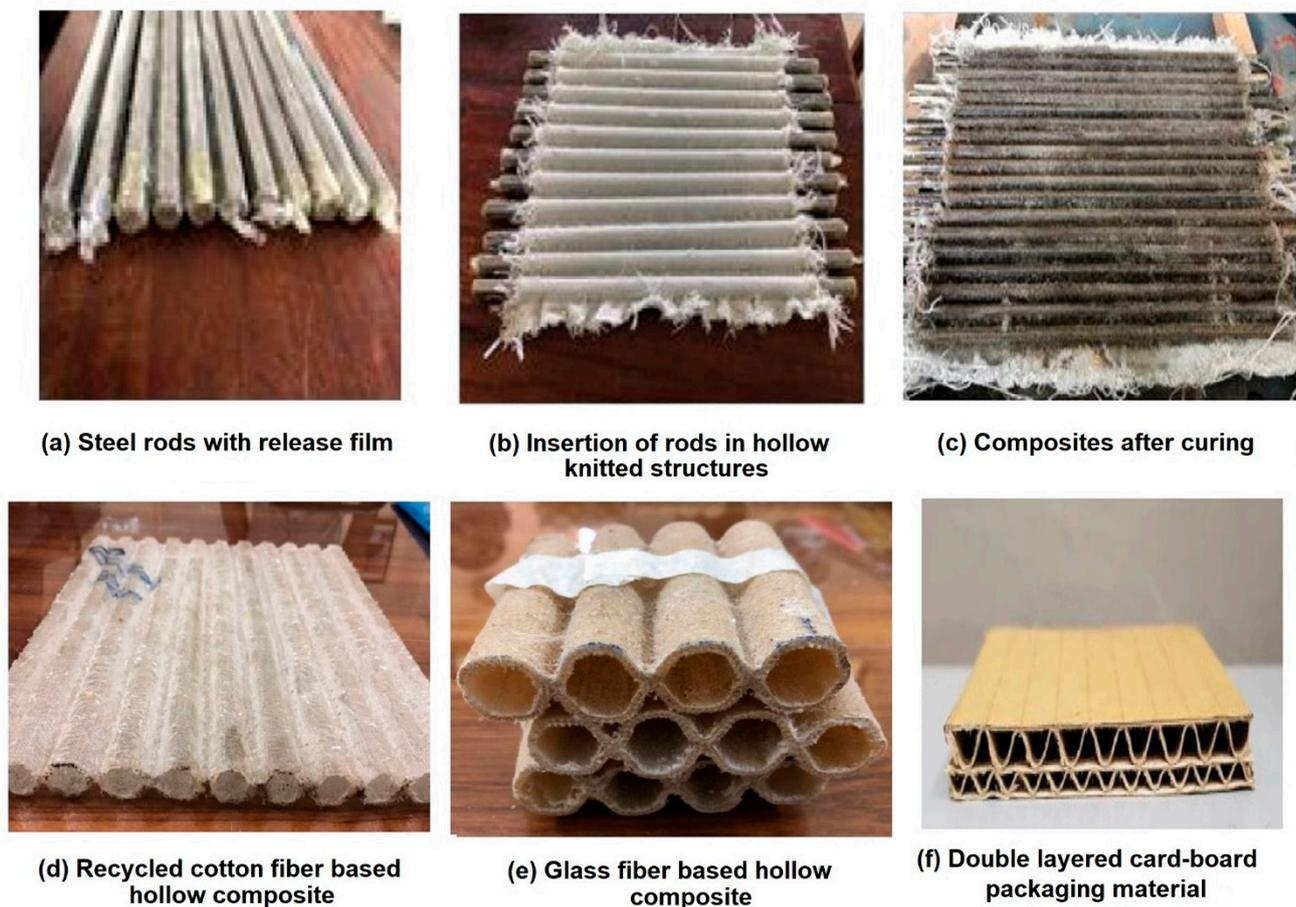
**Figure 2.** Photographs of developed composite samples versus double-layered cardboard.
