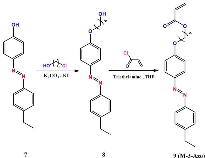
**Figure S3.** Scheme for synthesis of monomer M-3-Azo.
