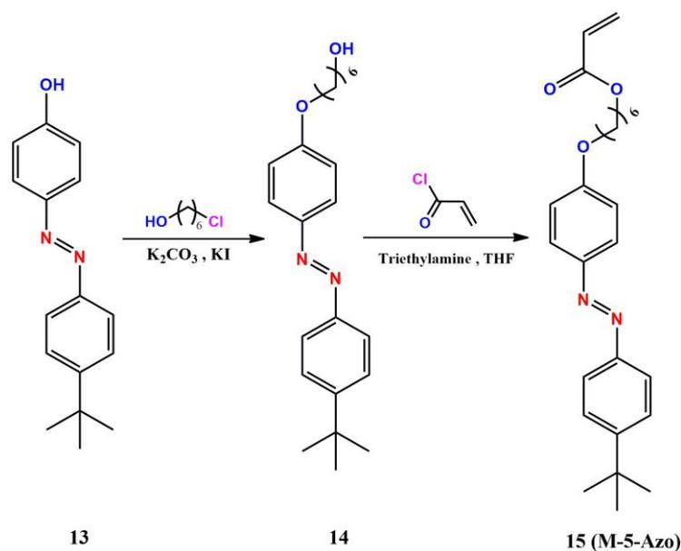
**Figure S5.** Scheme for synthesis of monomer M-5-Azo.
