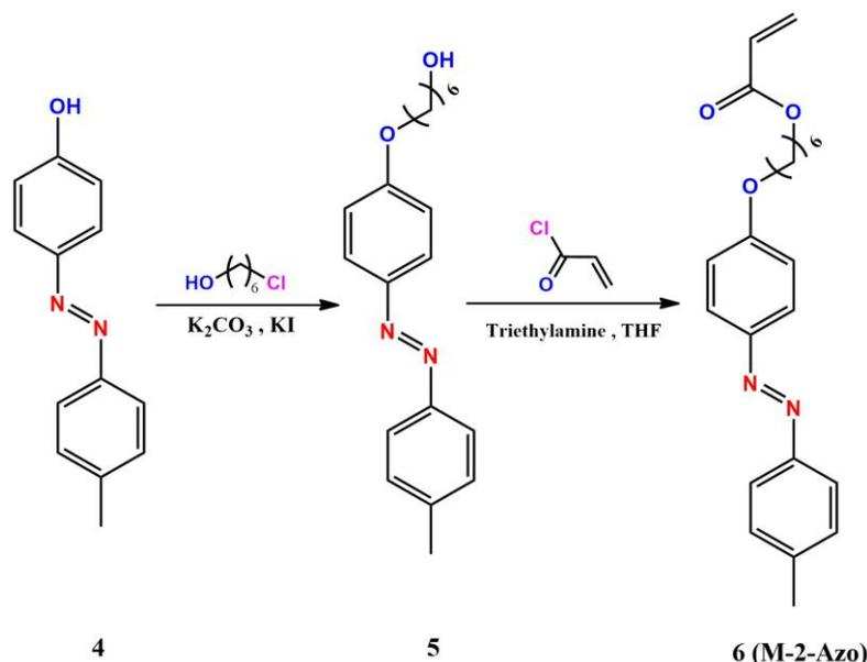
**Figure S2.** Scheme for synthesis of monomer M-2-Azo.
