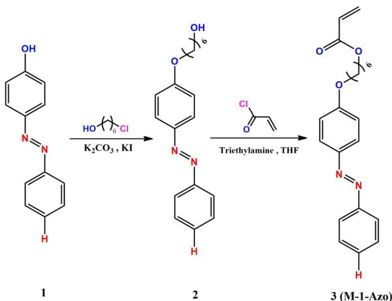
**Figure S1.** Scheme for synthesis of monomer M-1-Azo.
