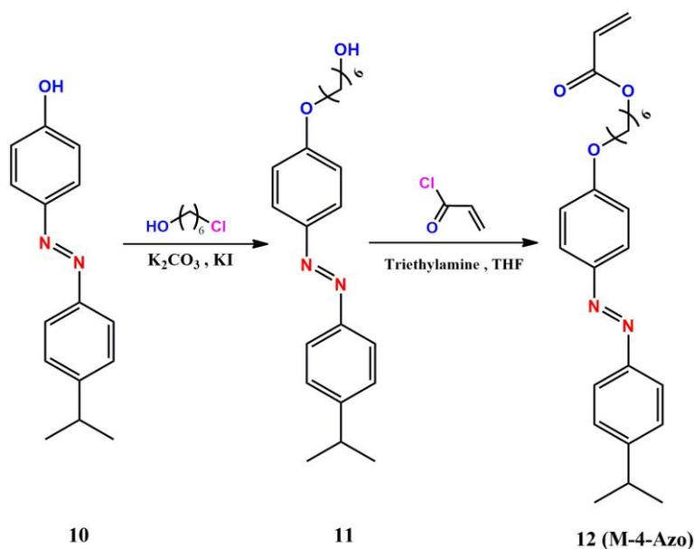
**Figure S4.** Scheme for synthesis of monomer M-4-Azo.
