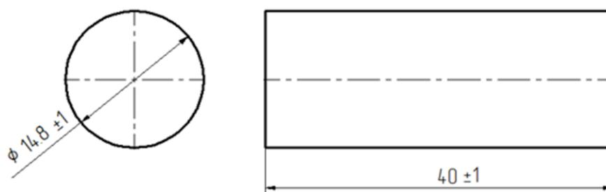
**Figure 1.** Dimensions [mm] of adhesives sample.
