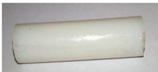
**Figure 2.** Specimens of E5/Z-1/100:12 epoxy compound after milling procedure.
