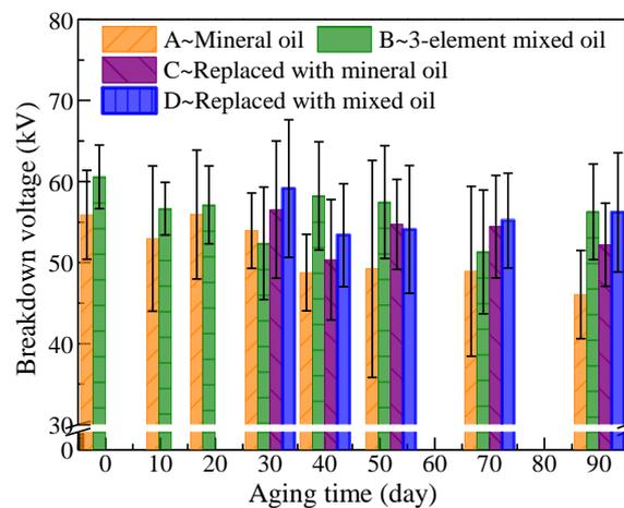
Figure 12. Breakdown voltage of insulation oil during the aging process.
