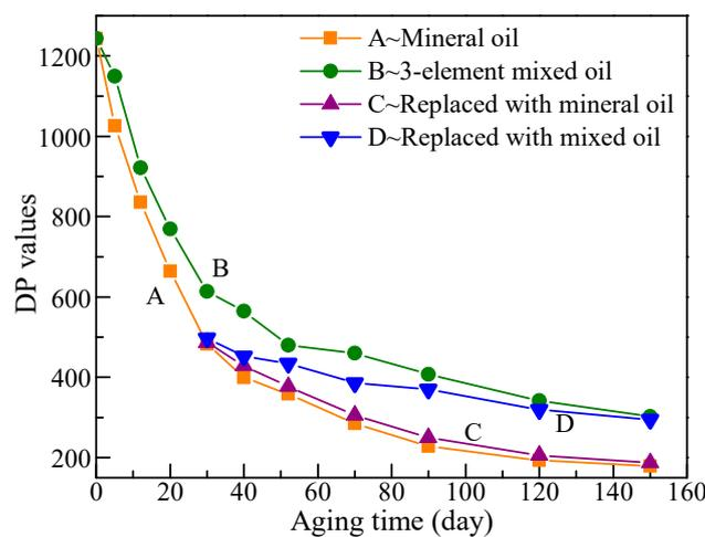
Figure 2. Test results of degree of polymerization (DP) values during the aging process.
