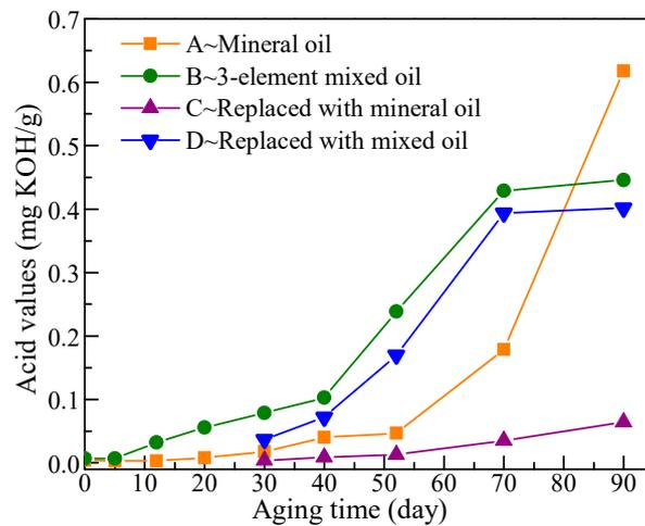
Figure 11. Acid values of insulation oils during the aging process.
