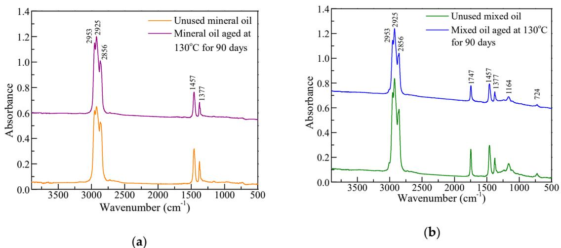
**Figure 8.** ATR-FTIR spectra of unused and aged insulation oils: (a) mineral oil; (b) three-element mixed oil.
