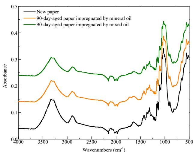
**Figure 3.** Attenuated total reflectance Fourier-transform infrared spectrometry (ATR-FTIR) of new paper and 90-day-aged cellulose paper.
