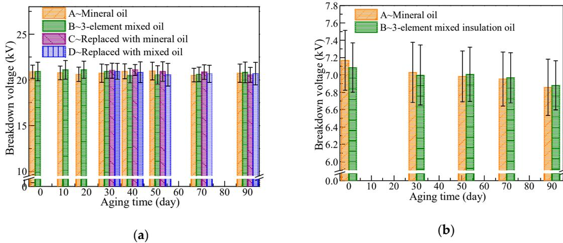
**Figure 7.** Breakdown voltage of cellulose polymers impregnated with different oils: (a) cellulose pressboard; (b) cellulose paper.
