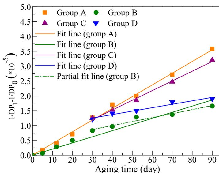
Figure 4. Test result of DP values during the aging process.
