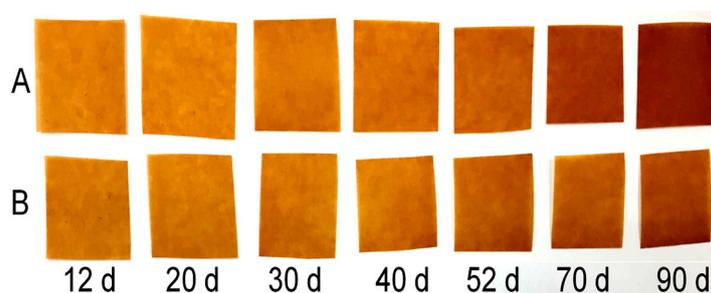
**Figure 6.** Colour of aged cellulose paper impregnated with mineral oil and mixed insulation oil: (A) cellulose paper impregnated with mineral oil; (B) cellulose paper impregnated with mixed oil.
