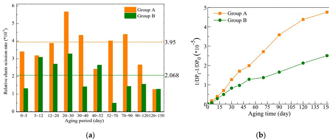
**Figure 5.** Relative chain-scission rate of cellulose in each aging period: (a) calculated  $k_{t_1 \sim t_2}$ ; (b) slope of the family of two points for Groups A and B.
