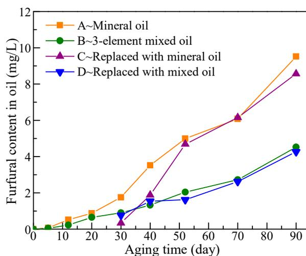
**Figure 9.** Furfural content in oil during aging process.
