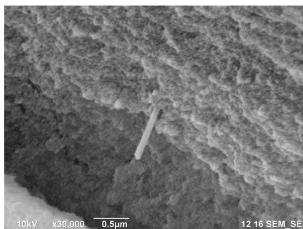
**Figure 7.** SEM micrograph of the silica gel with 0.05% halloysite cleaved in liquid nitrogen. The halloysite nanotube is visible in the center of the image. Scale bar, 500 nm.
