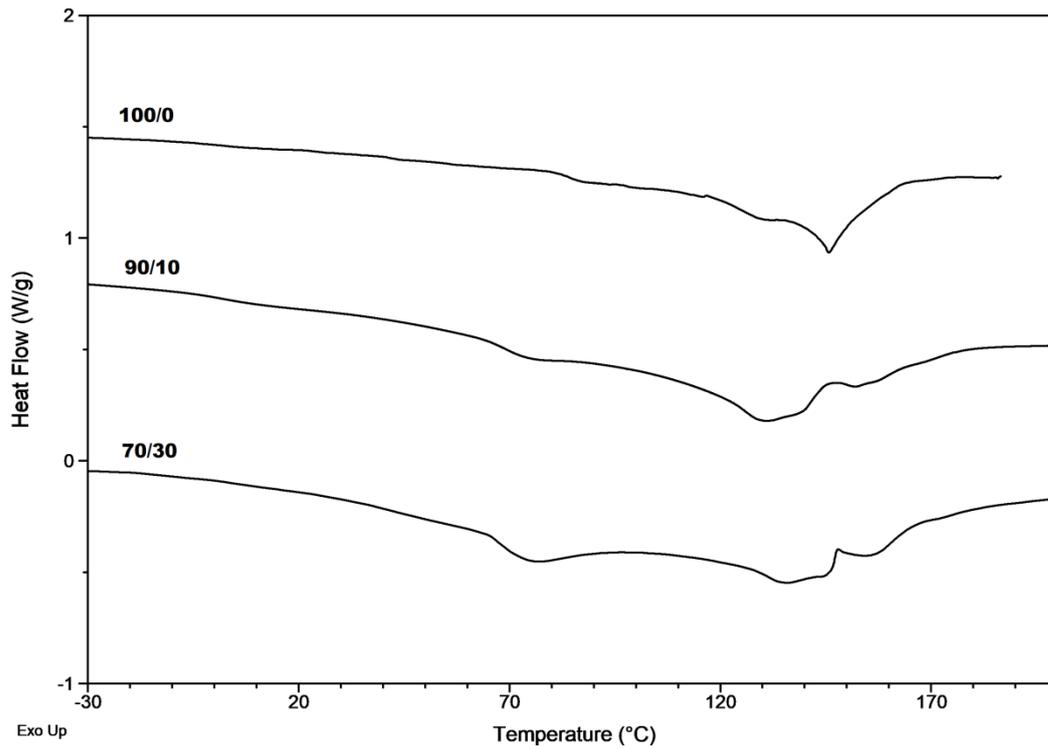
DSC plot of P(3HB-co-4HB)/cork composites (100/0), (90/10), (70/30) after 21 days of degradation in the BIODEGMA.
