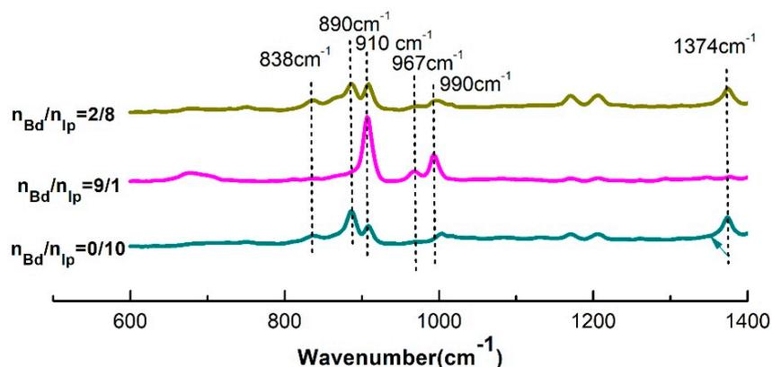
**Figure 9.** FTIR spectra of the resulting copolymers fabricated by coordination polymerization at the Bd:Ip mole ratios of 2:8, 9:1 and 0:10, respectively. Polymerization conditions: TNPP:Mo = 6,  $[M] = 0.18 \text{ g}\cdot\text{mL}^{-1}$ , Al:Mo = 5,  $T = 60 \text{ }^\circ\text{C}$ , Mo:[M] =  $8 \times 10^{-4}$ ,  $t = 7 \text{ h}$ .
