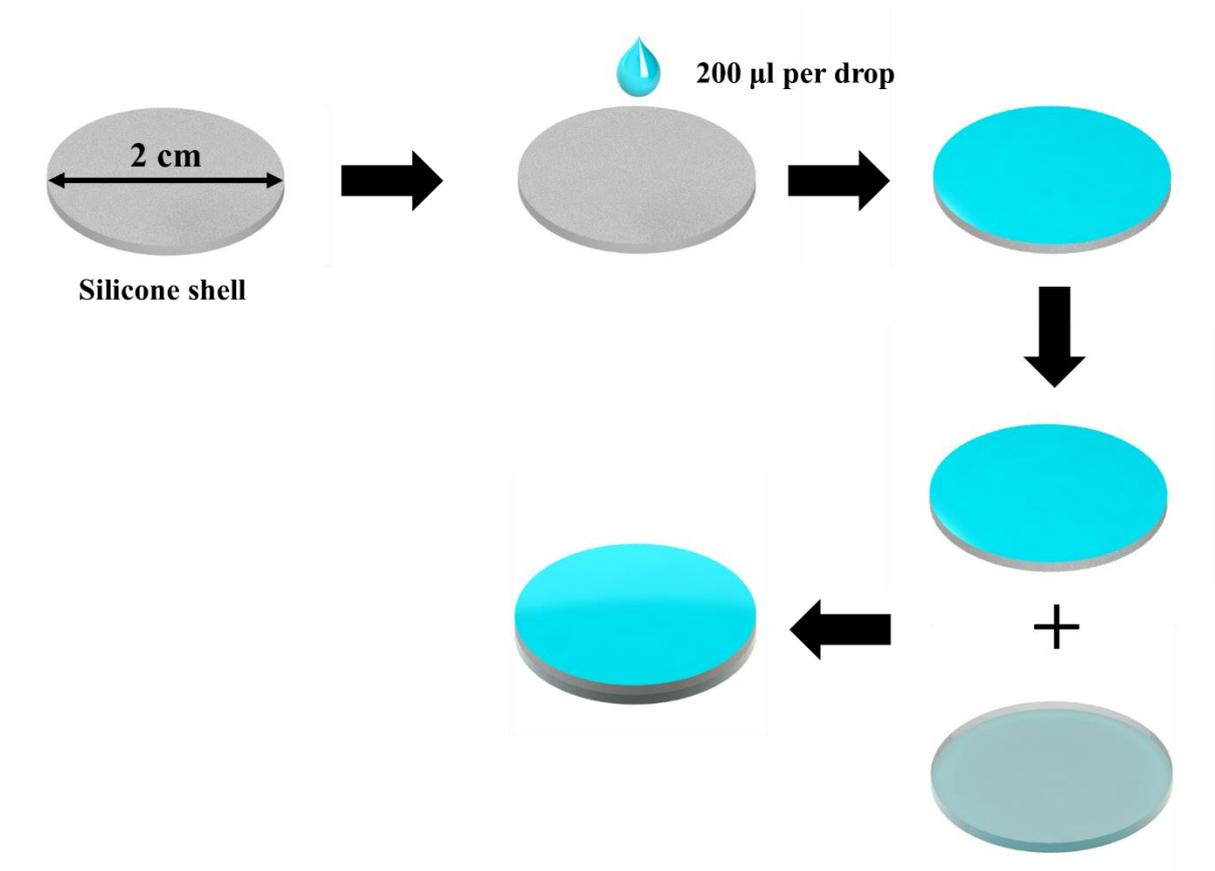
**Figure S1.** Schematic of the preparation of the entire coating on the surface of the implant shell.
