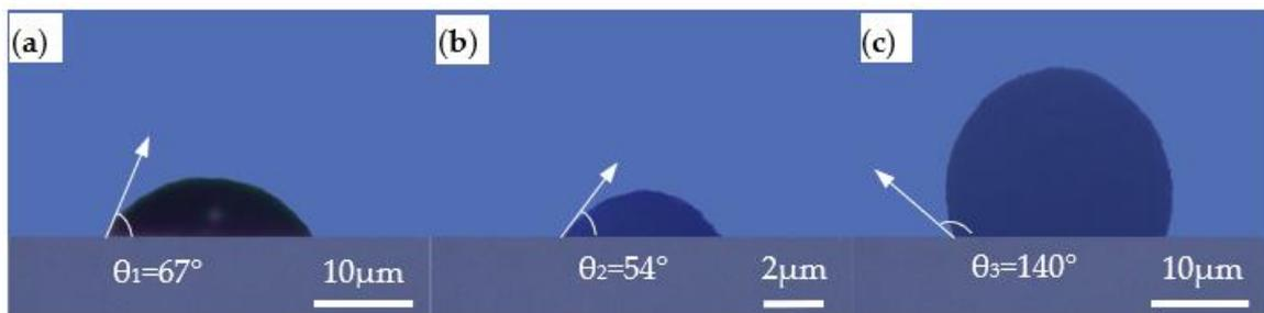
Figure 9. Contact angles of different materials at 20 °C: (a) MC-Wax; (b) PCL; (c) PMMA.
