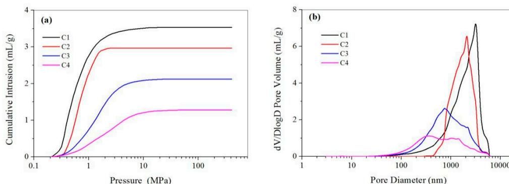
**Figure 10.** (a) Cumulative mercury intrusion traces and (b) pore size distribution of the CMC/CA microspheres fabricated with Cu(II) content of 25mM (C1), 50mM (C2), 100mM (C3), and 200mM (C4) in the outer aqueous solution.
