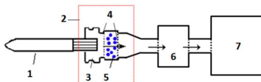
**Figure 2.** Device to simulate the addition of absorbents to the cigarette filter. (1) cigarette, (2) homemade device, (3) cigarette holder, (4) 120 mesh sieve, (5) sample, (6) Cambridge filter pad, and (7) smoking machine.
