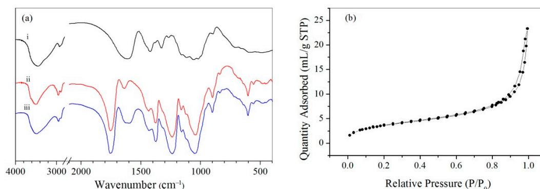
**Figure 3.** (a) FTIR of CMC (i), CA (ii), and CMC/CA microspheres (iii). (b) Typical nitrogen adsorption curves of CMC/CA microspheres.
