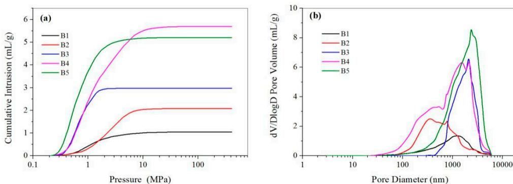
**Figure 8.** (a) Cumulative mercury intrusion traces and (b) pore size distribution of the CMC/CA microspheres fabricated with W1/O ratios of 10/100 (B1), 30/100 (B2), 50/100 (B3), 70/100 (B4), and 90/100 (B5).
