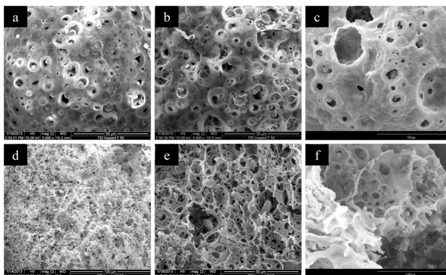
**Figure 5.** The SEM images of CMC/CA microspheres fabricated with 2% (a,d), 3% (b,e), 4% (c,f) CMC concentrations. Images (a–c) were the surface images while (d–f) were the cross-section images of CMC/CA microspheres.
