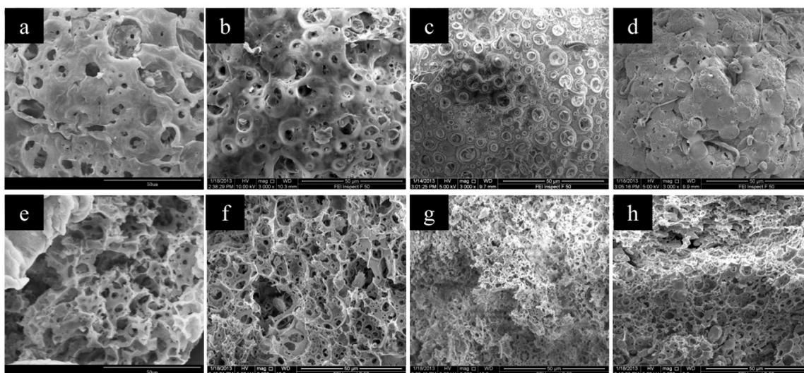
**Figure 9.** The SEM images of CMC/CA microspheres fabricated with Cu(II) content of 25mM (a,e), 50mM (b,f), 100mM (c,g), 200mM (d,h) in the outer aqueous solution. Images (a–d) are the surface images while (e–h) are the cross-section images of the CMC/CA microspheres.
