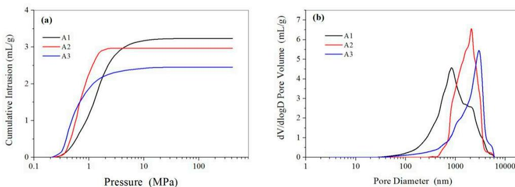
**Figure 6.** (a) Cumulative mercury intrusion traces and (b) pore size distribution of the CMC/CA microspheres fabricated with 2% (A1), 3% (A2), 4% (A3) CMC concentration.
