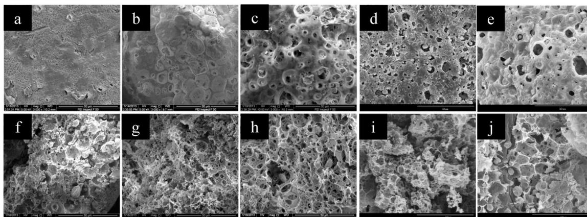
**Figure 7.** The SEM images of CMC/CA microspheres fabricated with W1/O ratios of 10/100 (a,f), 30/100 (b,g), 50/100 (c,h), 70/100 (d,i), and 90/100 (e,j). Images (a–e) were the surface images while (f–j) were the cross-section images of the CMC/CA microspheres.
