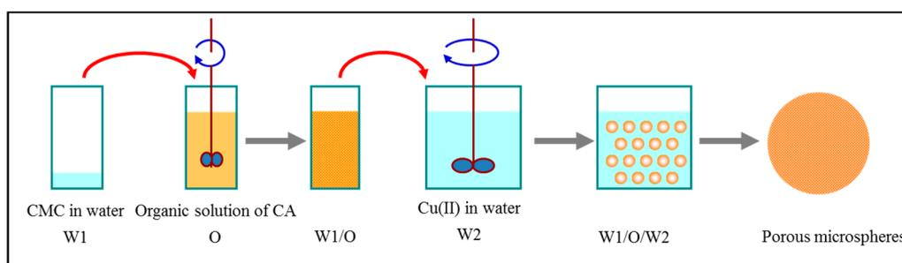
**Figure 1.** Synthesis pathway of CMC/CA microspheres.
