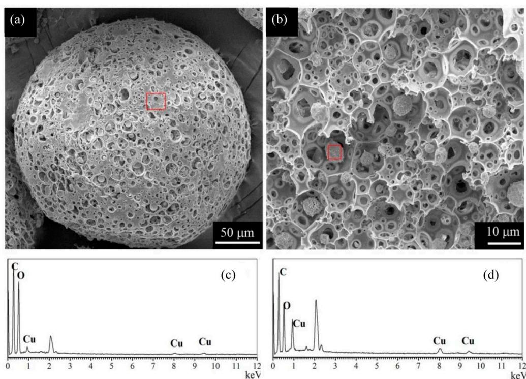
**Figure 4.** (a,b) SEM images of CMC/CA microsphere. (c,d) The corresponding EDS spectra of CMC/CA microsphere. (a,c) denotes the surface structure while (b,d) were the cross-section structure of the microspheres.
