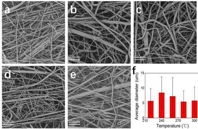
**Figure 1** SEM graphs of the PP fiber prepared by meltblown under different melt temperatures. 220°C (a), 240°C (b), 260°C (c), 280°C (d), 300°C (e). And the fiber diameter analysis of these fabrics (f).
