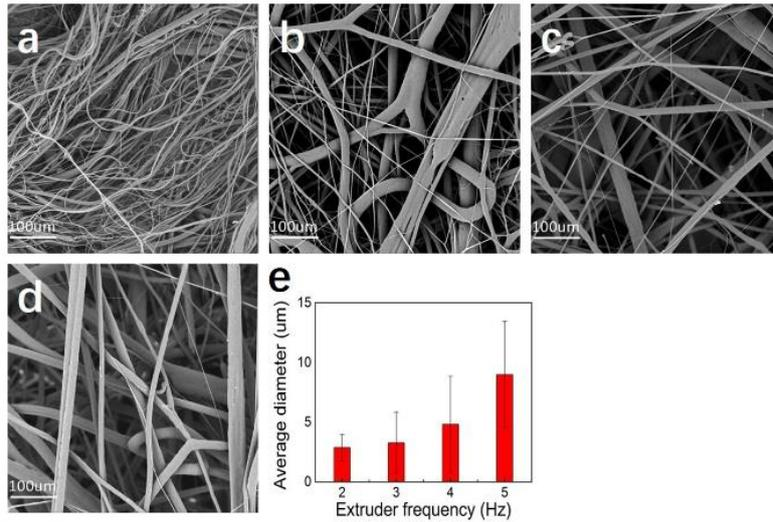
**Figure 3** SEM graphs of the PP fiber prepared by meltblown under different extruder screw rotating speeds. 2 Hz (120 rpm) (a), 3Hz (180 rpm) (b), 4 Hz (240 rpm) (c), 5 Hz (300 rpm) (d). And the fiber diameter analysis of these fabrics (e).
