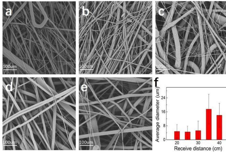
**Figure 5** SEM graphs of the PP fiber prepared by meltblown under different DCDs. 20 cm (a), 25 cm (b), 30 cm (c), 35 cm (d), 40 cm (e). And the fiber diameter analysis of these fabrics (f).
