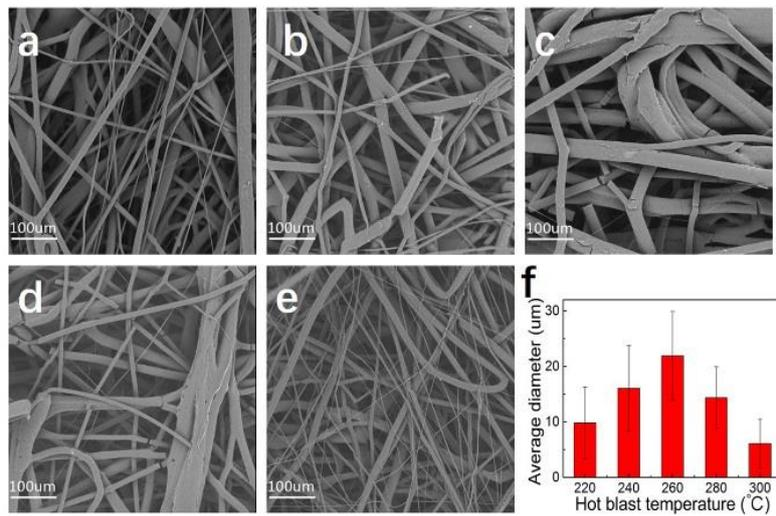
**Figure 2** SEM graphs of the PP fiber prepared by meltblown under different air temperatures. 220°C (a), 240°C (b), 260°C (c), 280°C (d), 300°C (e). And the fiber diameter analysis of these fabrics (f).
