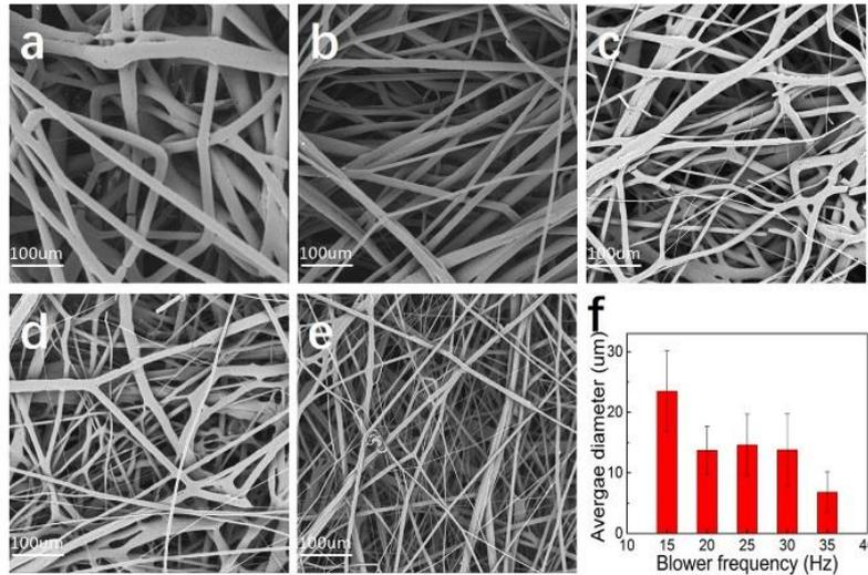
**Figure 4** SEM graphs of the PP fiber prepared by meltblown under different blower speeds. 15 Hz (90 rpm) (a), 20 Hz (1200 rpm) (b), 25 Hz (1500 rpm) (c), 30 Hz (1800 rpm) (d), 35 Hz (2100 rpm) (e). And the fiber diameter analysis of these fabrics (f).
