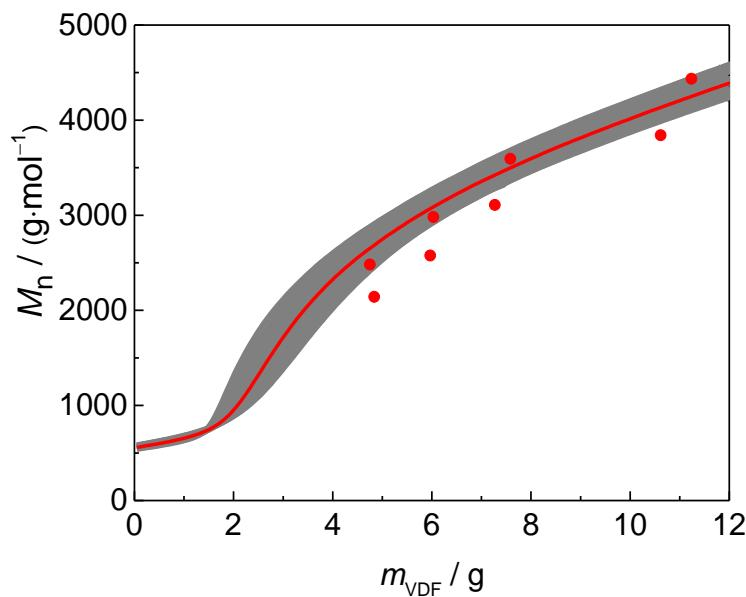
**Figure S2:** Sensitivity of the parameters  $C_{\text{tr}}$  and  $C_{\text{ex}}$ . The red line shows the simulation results with the optimum values and the red points the experimental data points (20 bar, 7.5 mmol I-C<sub>4</sub>F<sub>8</sub>-I (sample 5)). The grey band represents simulations carried out with 16 points taken from the outer sphere of the confidence interval, indicating that in all cases a good description of the experimental results is obtained.
