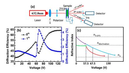
**Figure 3.** (a) Experiment setup for measuring the diffraction efficiency of the PS-SPLC grating. (b) Voltage dependent diffraction efficiencies of the zeroth and first orders. (c) Schematic diagram of the refractive index mismatch between the 3D twist spheres (3-DTSs) ( $n_{3-DTS}$ ) and the disclinations ( $n_{disclination}$ ).
