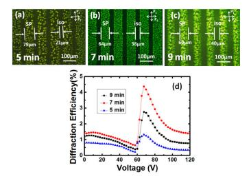
**Figure 6.** Monomer diffusion effect on the properties of the LC grating. (**a**–**c**) The polarizing micrographs of PS-SPLC grating with different diffusion time and (**d**) the diffraction efficiency on first order with different diffusion time.
