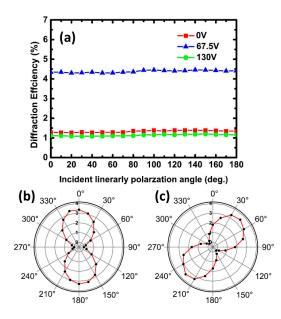
**Figure 4.** (a) The first order diffraction efficiency with different incident light polarization angles at applied voltages of V = 0 V, 67.5 V, and 130 V. (b,c) Polarization of first order diffracted beam with  $0^{\circ}$  and  $45^{\circ}$  polarized incident light at 67.5 V, respectively.
