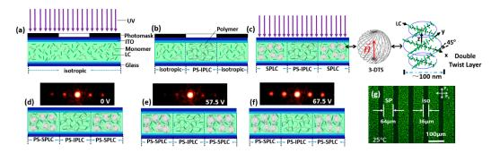
**Figure 2.** (**a**–**c**) Schematic diagram of the polymer-stabilized sphere phase liquid crystal (PS-SPLC) grating fabrication process. Diffraction pattern and possible schematic diagram of liquid crystalline molecular orientation of the PS-SPLC grating at (**d**) V = 0 V, (**e**) 57.5 V, and (**f**) 67.5 V. (**g**) the polarizing micrographs of PS-SPLC grating in reflection mode at the turn-off state.
