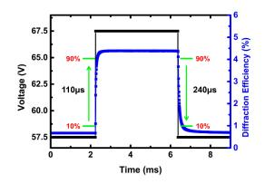
**Figure 5.** Plots the electro-optical response of rise time and decay time of the liquid crystal (LC) grating on first order.
