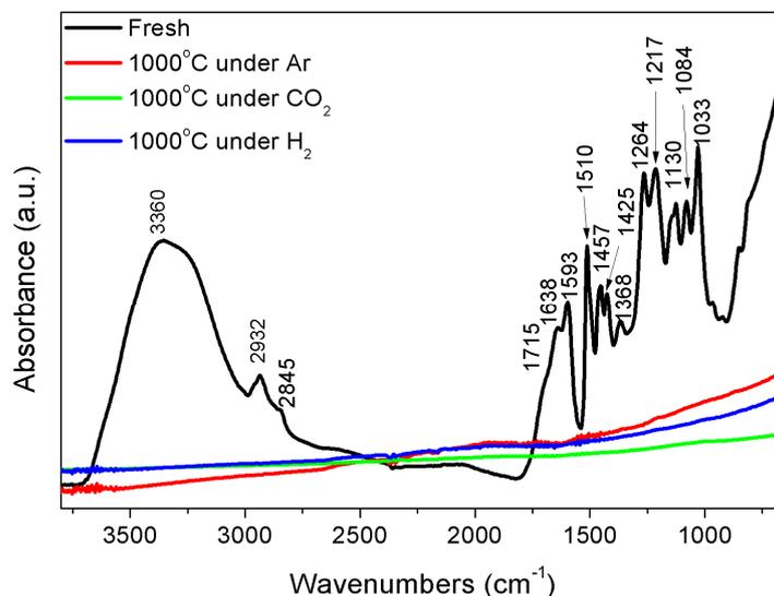
Figure 1. FTIR spectrum of raw and thermally decomposed kraft lignin.
