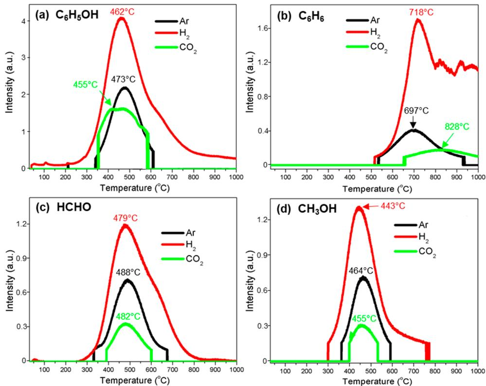
**Figure 4.** Gas evolution profiles of the thermal decomposition of kraft lignin under argon (Ar), hydrogen (H<sub>2</sub>), and carbon dioxide (CO<sub>2</sub>) atmospheres: (a) C<sub>6</sub>H<sub>5</sub>OH; (b) C<sub>6</sub>H<sub>6</sub>; (c) HCHO; and (d) CH<sub>3</sub>OH.
