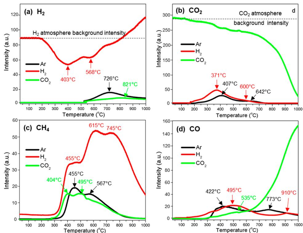
**Figure 3.** Gas evolution profiles of the thermal decomposition of kraft lignin under argon (Ar), hydrogen (H<sub>2</sub>), and carbon dioxide (CO<sub>2</sub>) atmospheres: (a) H<sub>2</sub>; (b) CO<sub>2</sub>; (c) CH<sub>4</sub>; and (d) CO.
