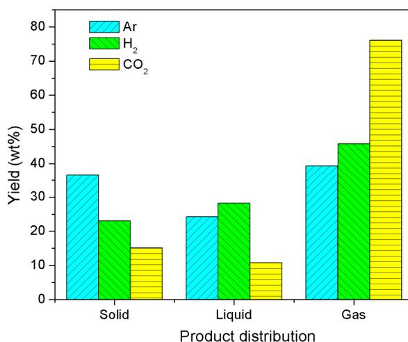
Figure 2. Products (solid carbon, liquid, and noncondensable gas) distribution of kraft lignin thermally decomposed using three different atmospheres at 1000 °C for 1 h.
