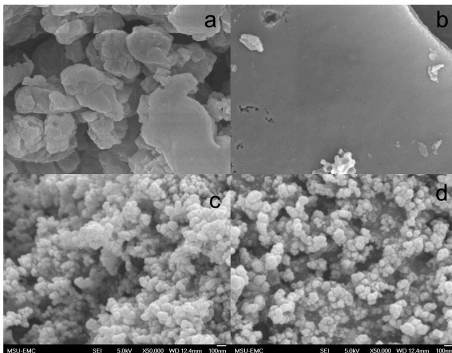
**Figure 6.** SEM images of raw kraft lignin (a) and solid products of kraft lignin thermally decomposed at  $1000^\circ\text{C}$  under three different atmospheres of Ar (b),  $\text{CO}_2$  (c), and  $\text{H}_2$  (d).
