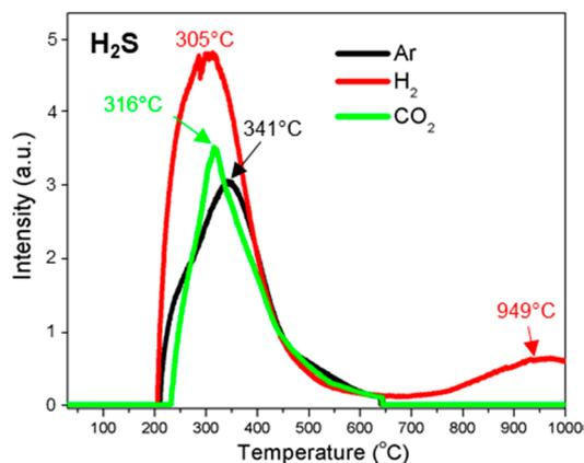
**Figure 5.** H<sub>2</sub>S evolution profiles of the thermal decomposition of kraft lignin under argon (Ar), hydrogen (H<sub>2</sub>), and carbon dioxide (CO<sub>2</sub>) atmospheres.
