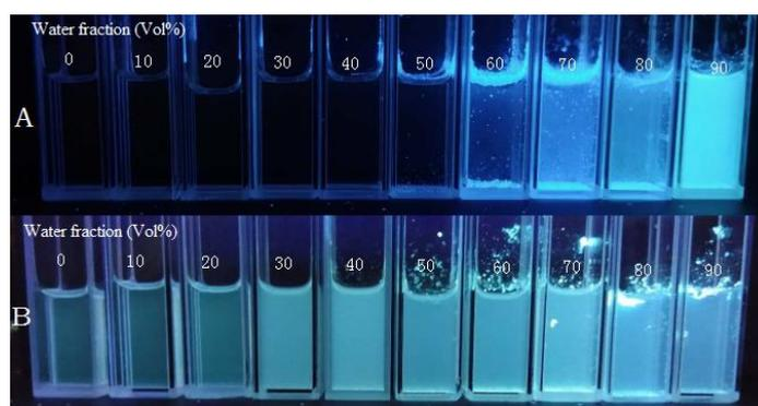
**Figure 4.** Comparison of fluorescence behaviors of (A) TPE ( $c_{\text{TPE}} = 2 \text{ mg/mL}$ ,  $6.0 \text{ } \mu\text{mol/mL}$ ) with (B) nanogel of  $\text{P}(\text{BPMA-}co\text{-ProHEMA})_{\text{gel-}b}\text{-PMMA}$  ( $c_{\text{nanogel}} = 1 \text{ mg/mL}$ ,  $c_{\text{TPE unit}} < 0.37 \text{ } \mu\text{mol/mL}$ ) in THF/water mixed solvents with different water fractions from 0% to 90%. UV light ( $\lambda = 365 \text{ nm}$ ) was used to excite emission.
