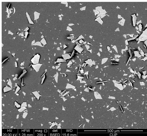
Figure 1. SEM images of three type micro glass flakes: (a) GF-B, (b) GF-M and (c) GF-S.
