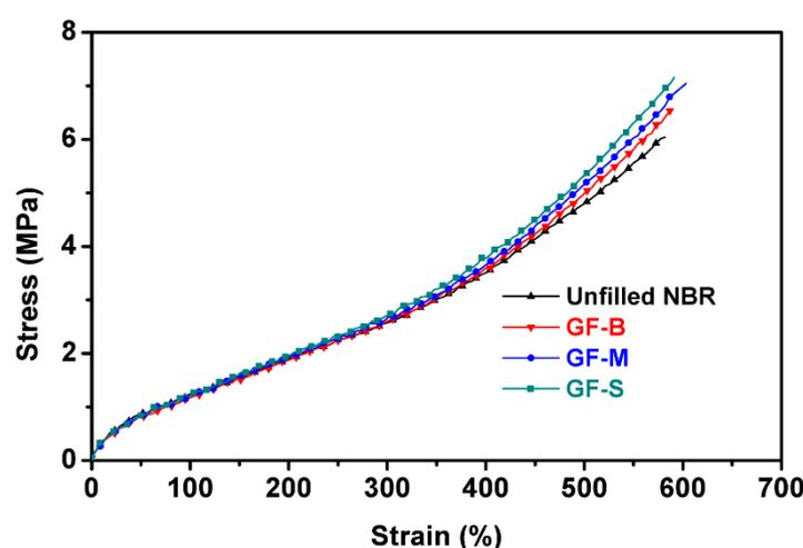
Figure 3. Stress-strain curves of sulphur-vulcanized NBR specimens.
