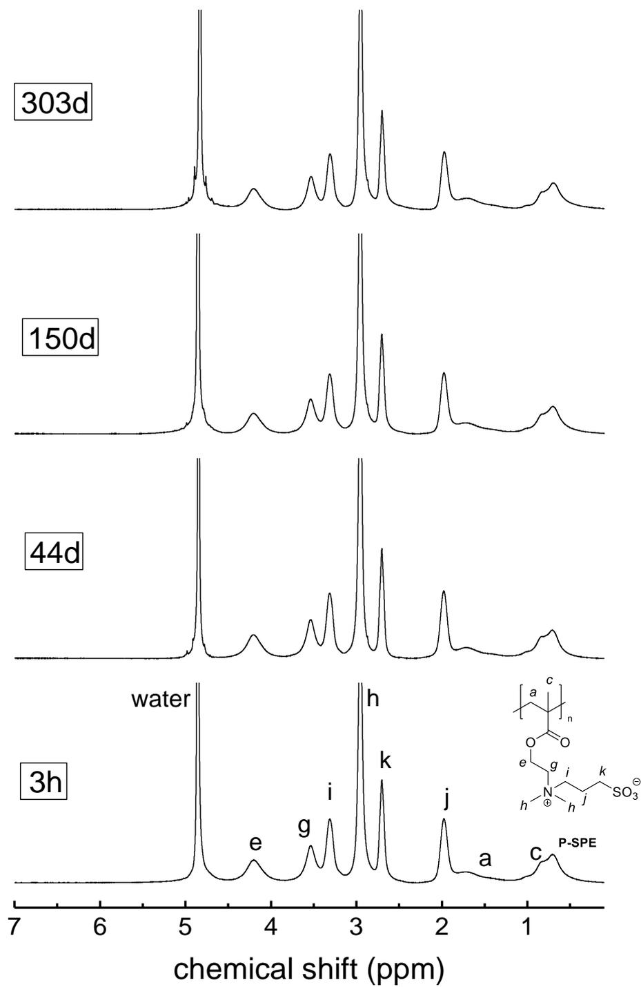
Figure S 84  $^1\text{H-NMR}$  spectrum showing the degradation of **P-SPE** in 1 M hydrochloric acid in  $\text{D}_2\text{O}$  (pH = 0) at room temperature over time.
