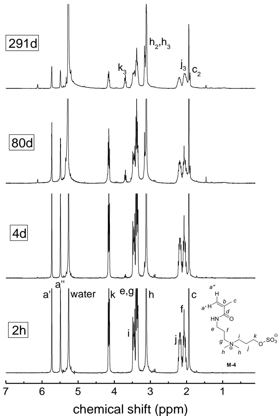
Figure S 39  $^1\text{H-NMR}$  spectrum showing the degradation of 0.1 M solution of **M-4** in hydrochloric acid in  $\text{D}_2\text{O}$  (pH = 0) at room temperature over time.
