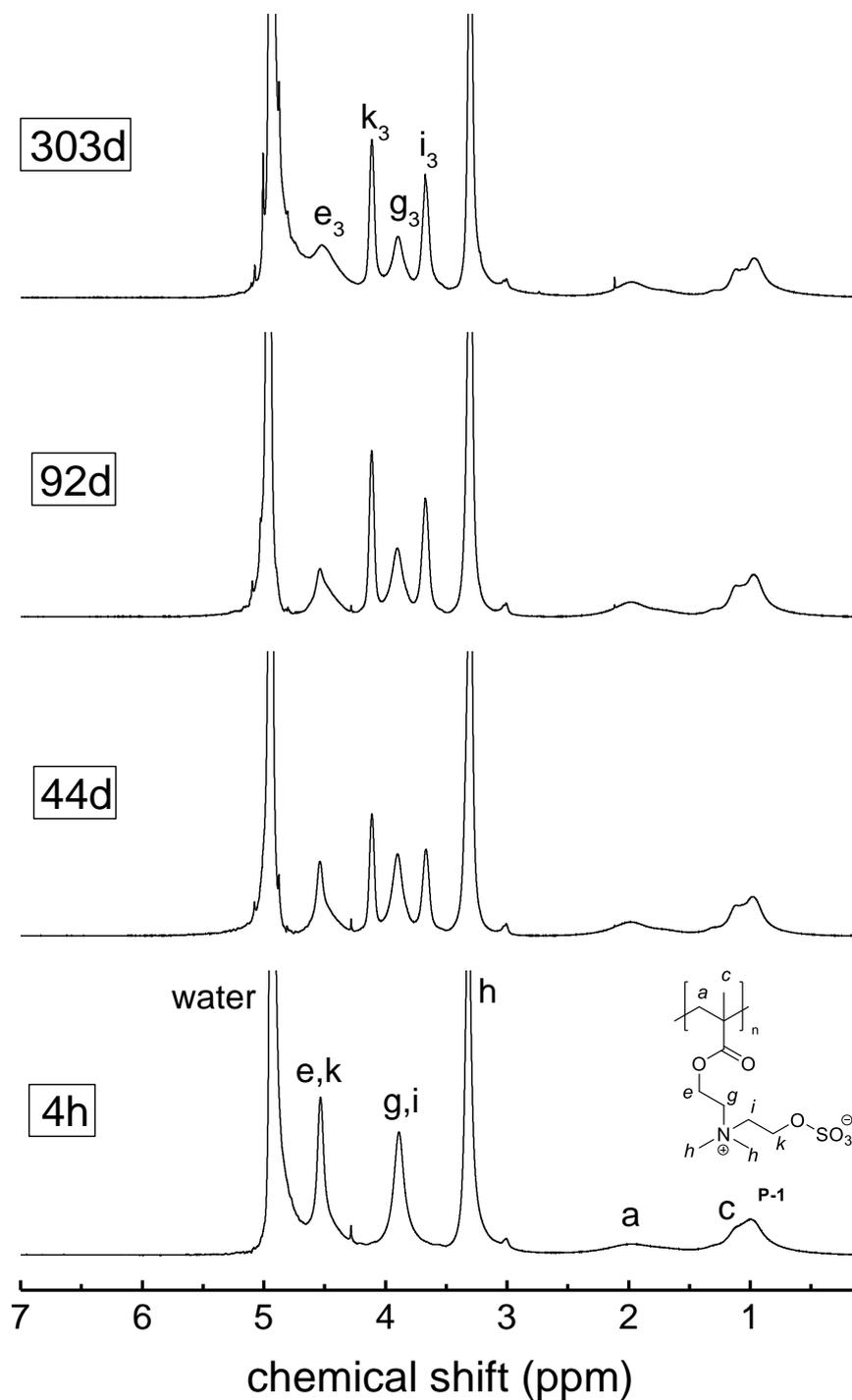
Figure S 86  $^1\text{H-NMR}$  spectrum showing the degradation of **P-1** in 1 M hydrochloric acid in  $\text{D}_2\text{O}$  ( $\text{pH} = 0$ ) saturated with sodium chloride at room temperature over time.
