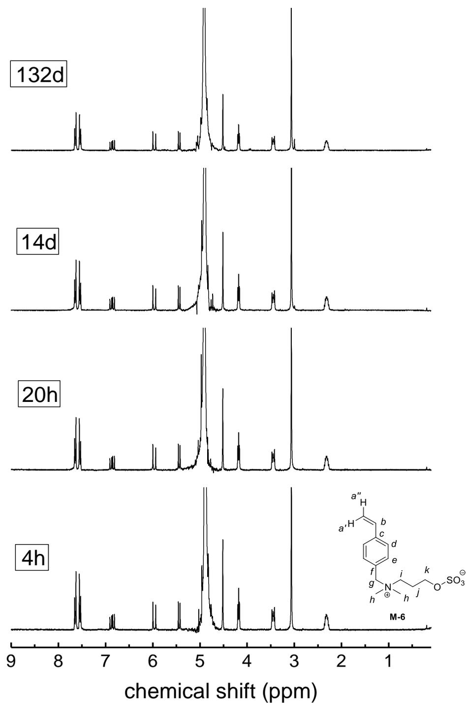
Figure S 69  $^1\text{H-NMR}$  spectrum showing the degradation of 0.1 M solution of **M-6** in sodium hydroxid in  $\text{D}_2\text{O}$  ( $\text{pH} = 14$ ) at room temperature over time.
