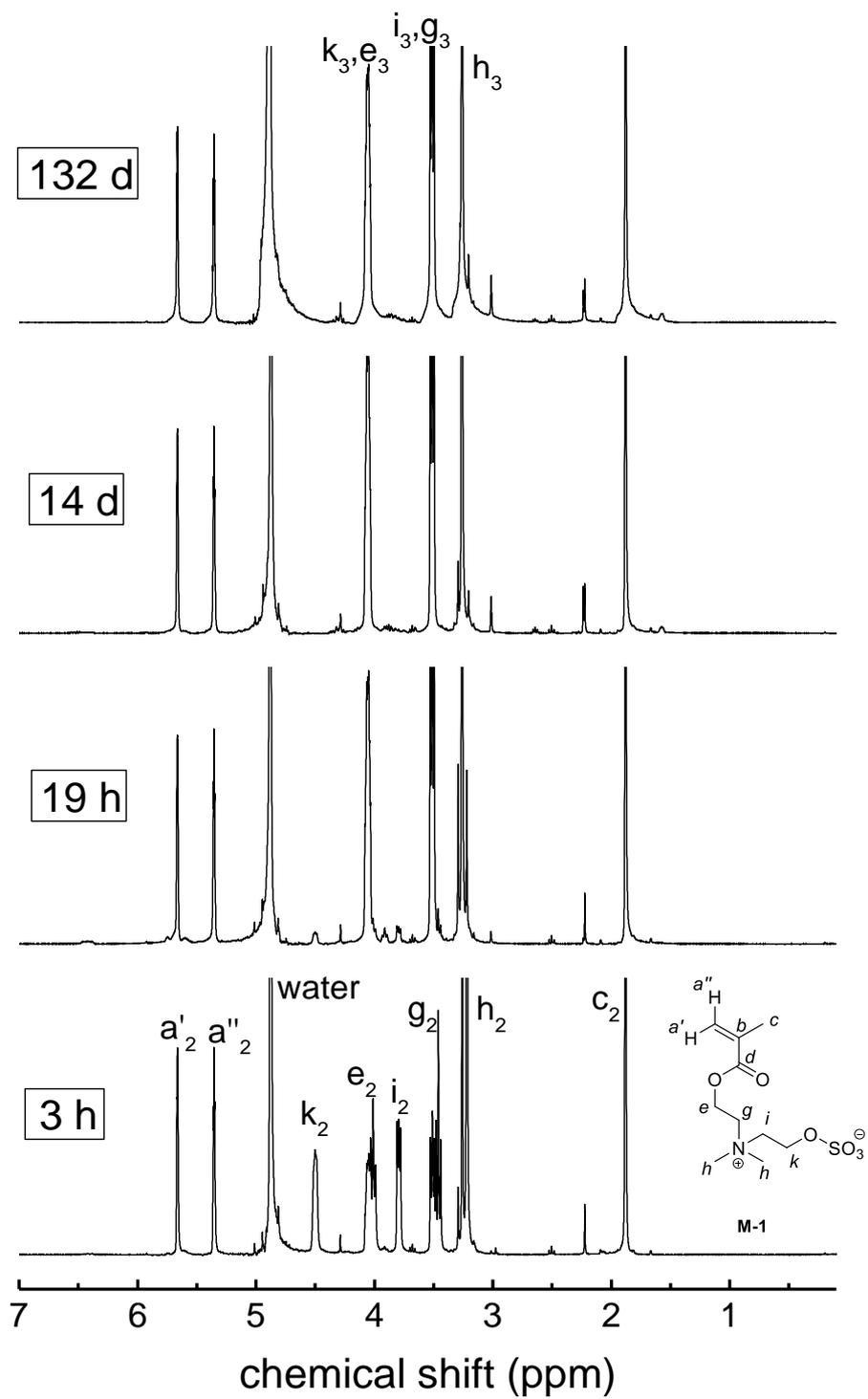
Figure S 64 <sup>1</sup>H-NMR spectrum showing the degradation of 0.1 M solution of **M-1** in sodium hydroxide in D<sub>2</sub>O (pH = 14) at room temperature over time.
