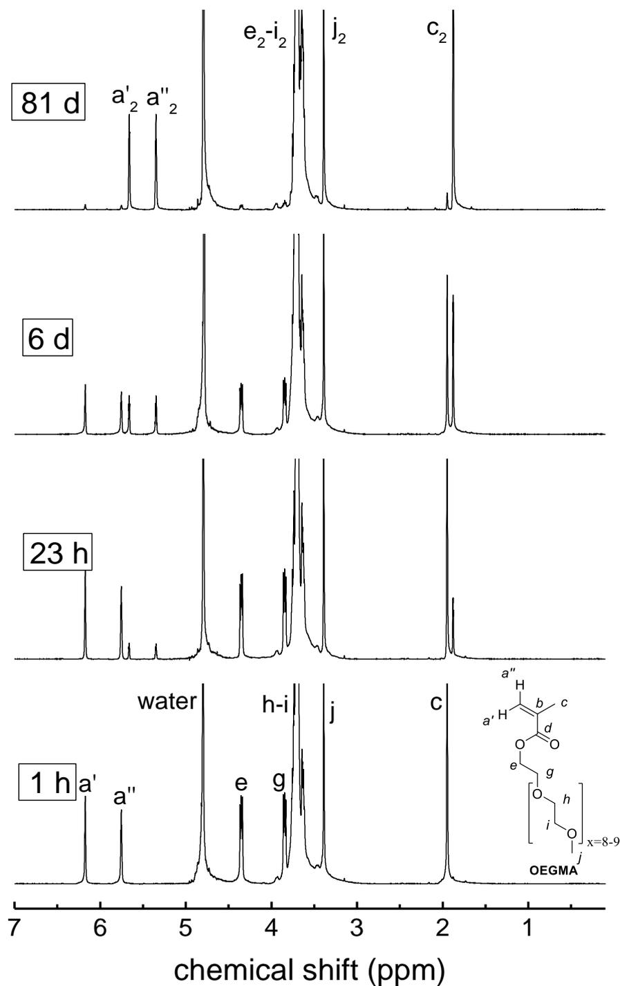
Figure S 50  $^1\text{H-NMR}$  spectrum showing the degradation of 0.1 M solution of OEGMA in carbonate buffer in  $\text{D}_2\text{O}$  (pH = 10) at room temperature over time.
