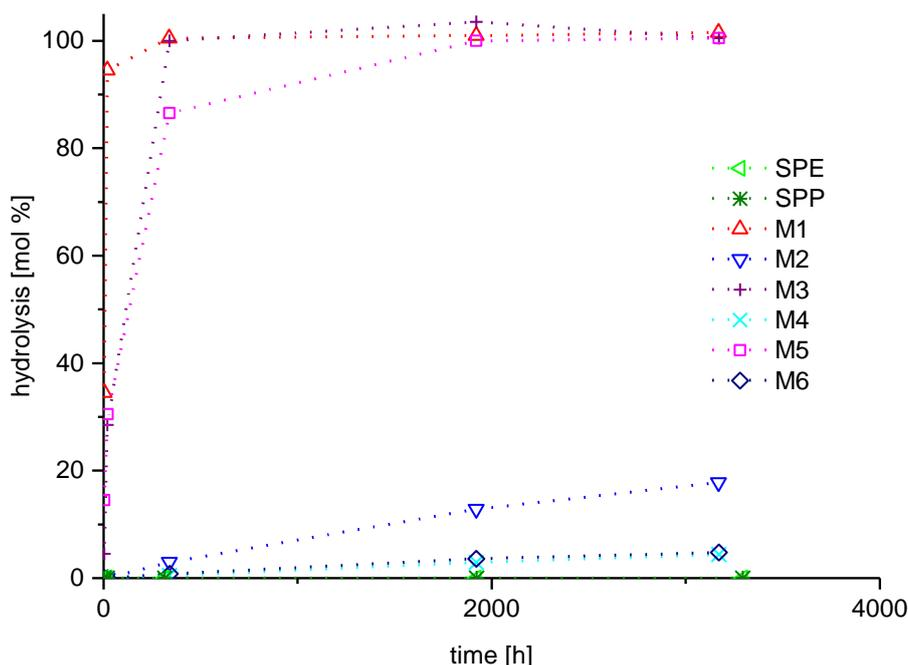
Figure S 60 Evolution of sulfate and sulfonate hydrolysis of monomers in sodium hydroxide in D<sub>2</sub>O (pH=14): (□) = **SPE**, (\*) = **SPP**, (△) = **M-1**, (▽) = **M-2**, (+) = **M-3**, (X) = **M-4**, (◻) = **M-5**, (◇) = **M-6**.
