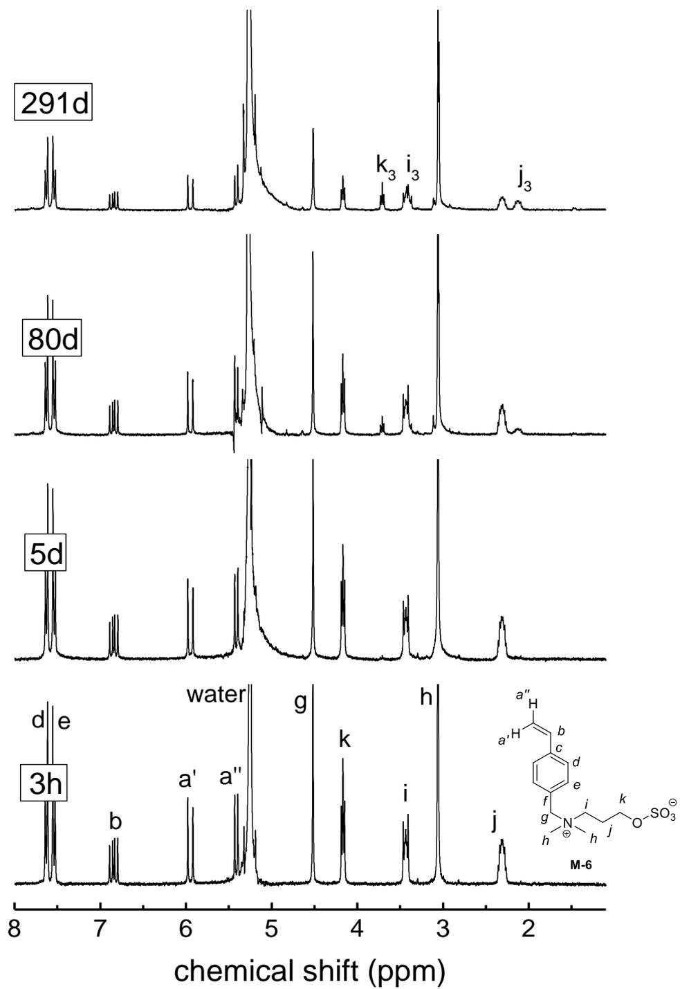
Figure S 41  $^1\text{H-NMR}$  spectrum showing the degradation of 0.1 M solution of **M-6** in hydrochloric acid in  $\text{D}_2\text{O}$  (pH = 0) at room temperature over time.
