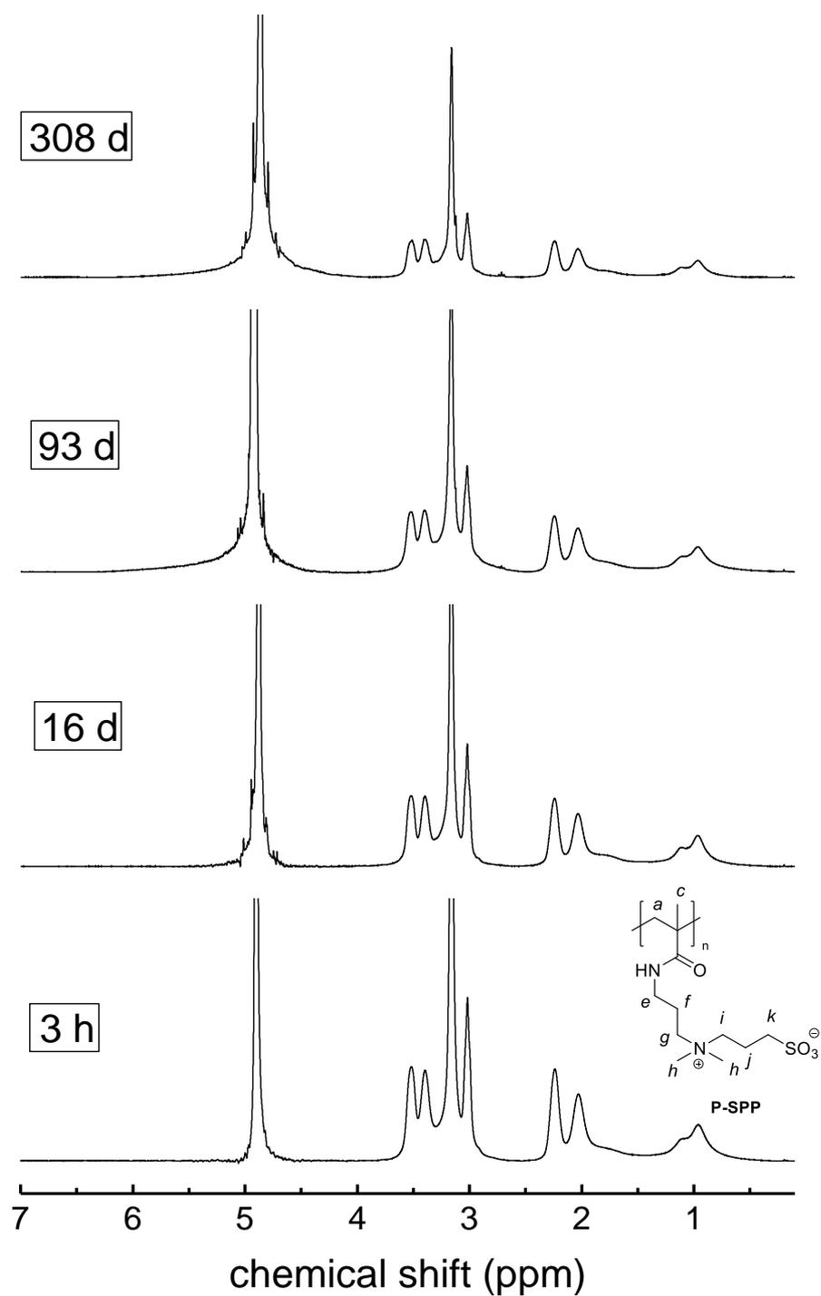
Figure S 97  $^1\text{H-NMR}$  spectrum showing the degradation of **P-SPP** in sodium hydroxide in  $\text{D}_2\text{O}$  (pH = 14) at room temperature over time.
