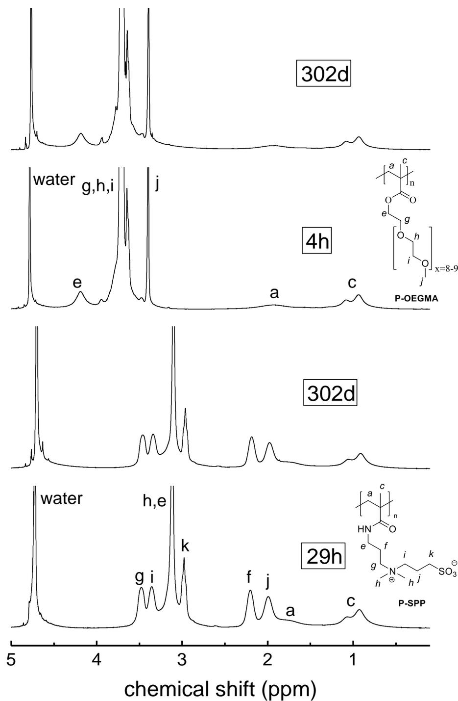
Figure S 91  $^1\text{H-NMR}$  spectrum showing the degradation of **P-OEGMA** and **P-SPP** in carbonate buffer in (pH = 10) at room temperature over time.
