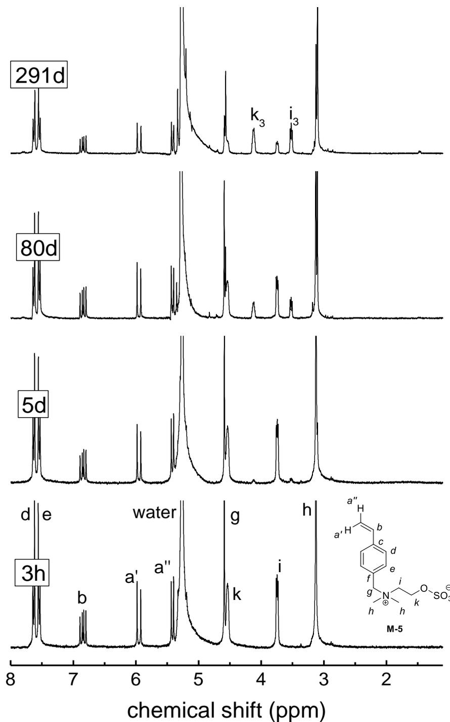
Figure S 40  $^1\text{H-NMR}$  spectrum showing the degradation of 0.1 M solution of **M-5** in hydrochloric acid in  $\text{D}_2\text{O}$  (pH = 0) at room temperature over time.
