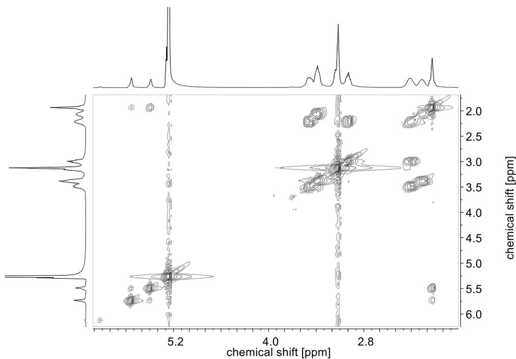
Figure S 42  $^1\text{H}$ - $^1\text{H}$ -COSY NMR spectra of 0.1 M solution of **SPP** in hydrochloric acid in  $\text{D}_2\text{O}$ , after 291 days.
