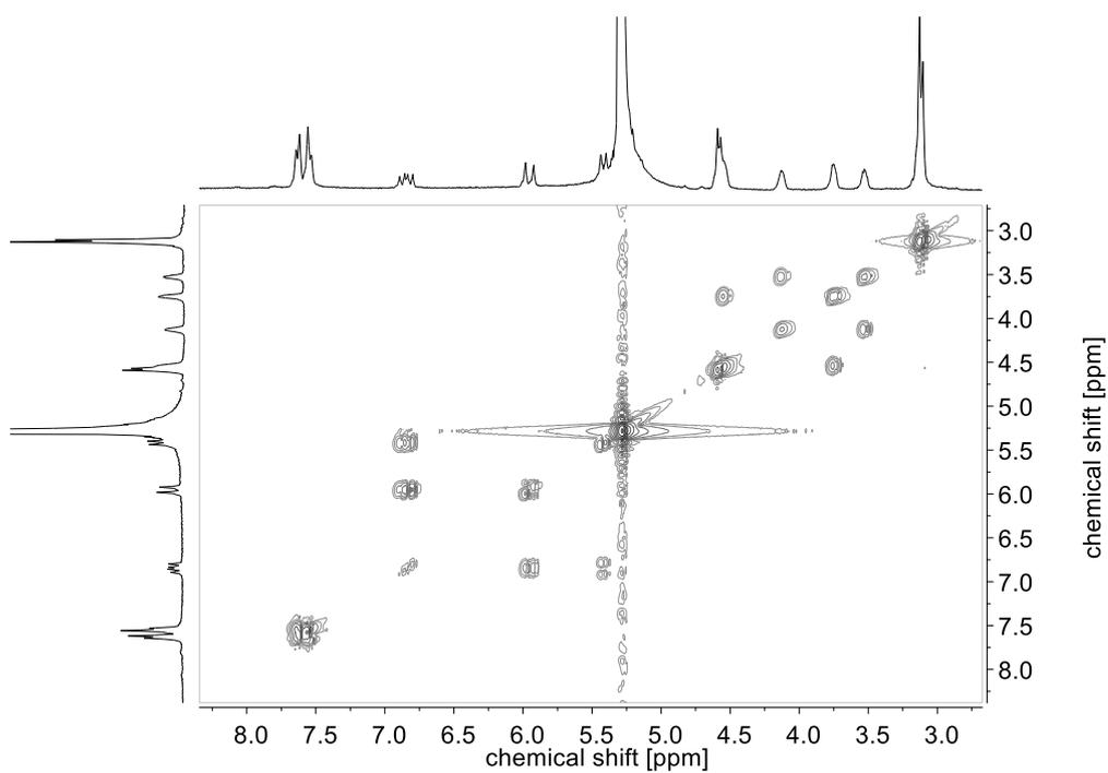
Figure S 47  $^1\text{H}$ - $^1\text{H}$ -COSY NMR spectra of 0.1 M solution of **M-5** in hydrochloric acid in  $\text{D}_2\text{O}$ , after 291 days.
