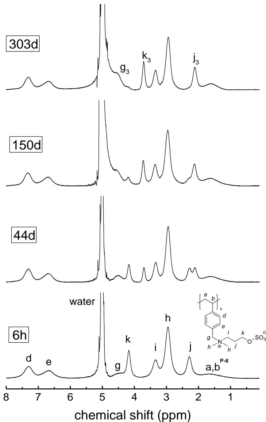
Figure S 90  $^1\text{H-NMR}$  spectrum showing the degradation of **P-6** in 1 M hydrochloric acid in  $\text{D}_2\text{O}$  (pH = 0) saturated with sodium chloride at room temperature over time.
