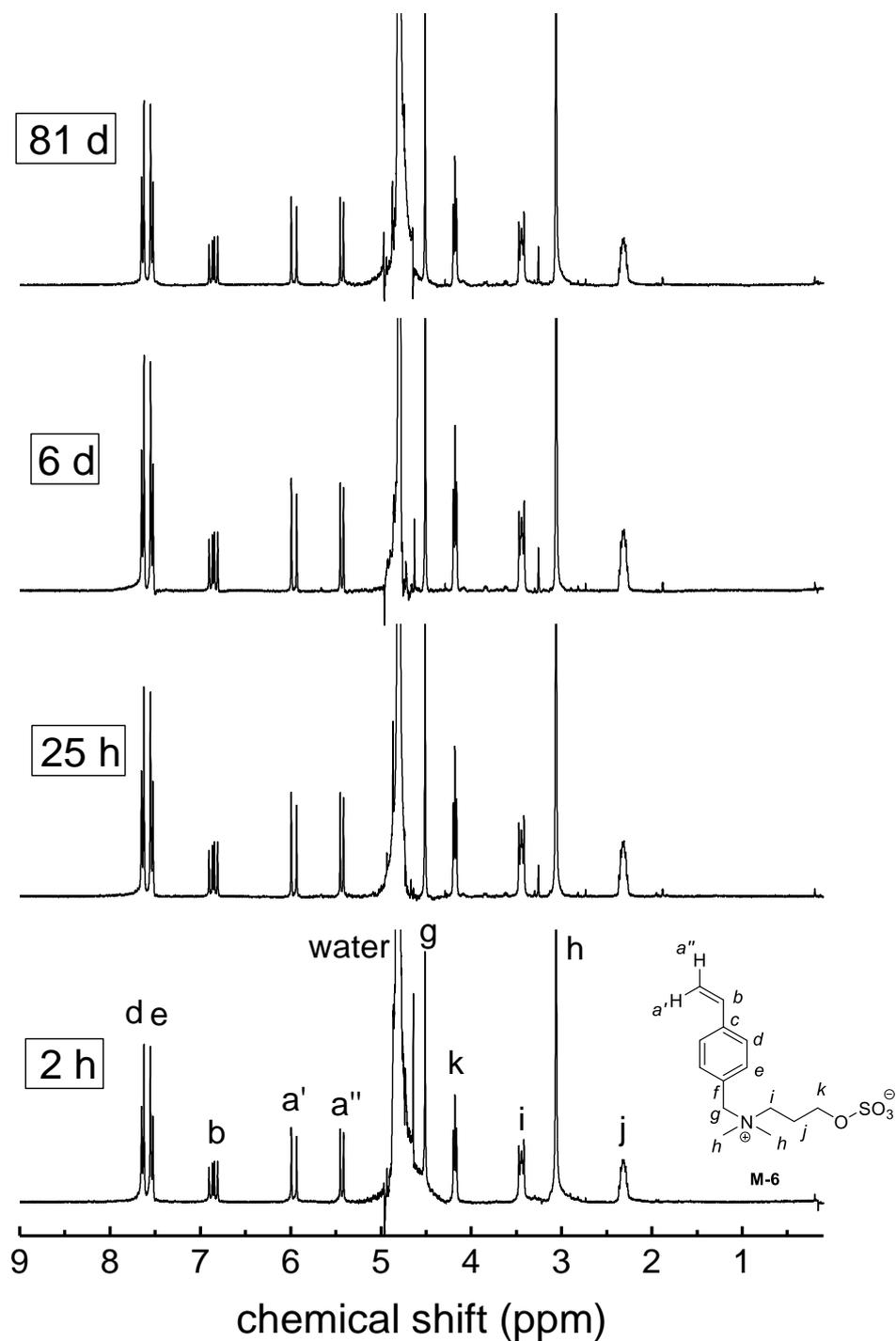
Figure S 58  $^1\text{H-NMR}$  spectrum showing the degradation of 0.1 M solution of **M-6** in carbonate buffer in  $\text{D}_2\text{O}$  (pH = 10) at room temperature over time.
