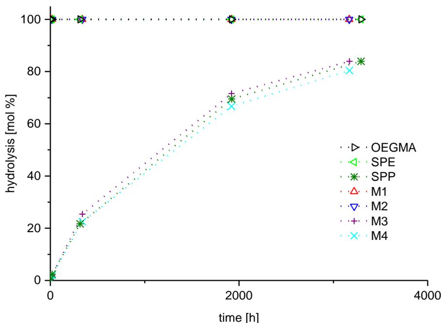
Figure S 59 Evolution of ester and amid hydrolysis of monomers in sodium hydroxide in D<sub>2</sub>O (pH=14): (□) = **OEGMA**, (□) = **SPE**, (\*) = **SPP**, (□) = **M-1**, (□) = **M-2**, (+) = **M-3**, (X) = **M-4**.
