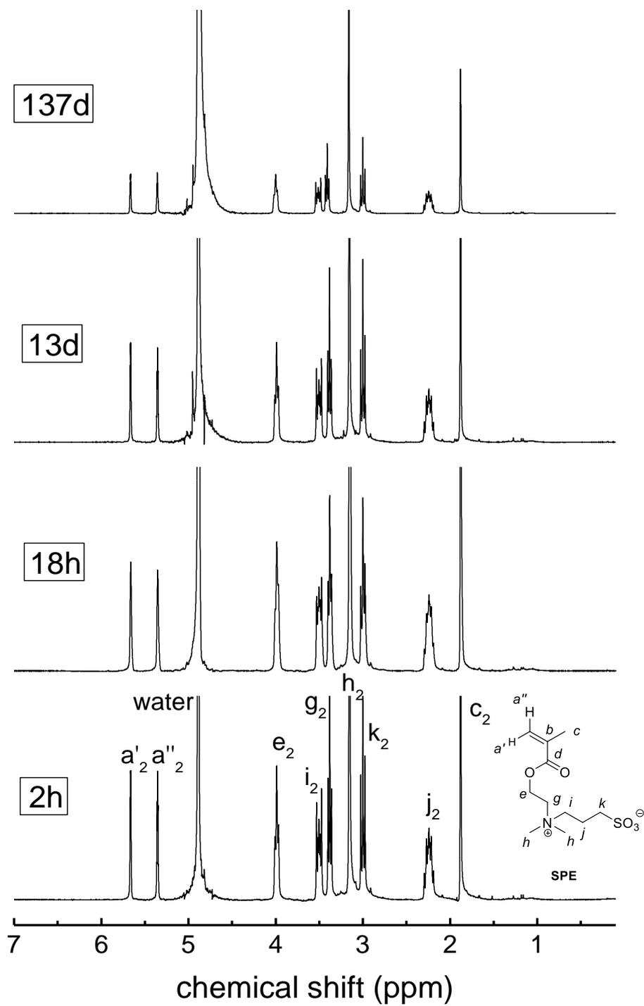
Figure S 62 <sup>1</sup>H-NMR spectrum showing the degradation of 0.1 M solution of **SPE** in sodium hydroxide in D<sub>2</sub>O (pH = 14) at room temperature over time.
