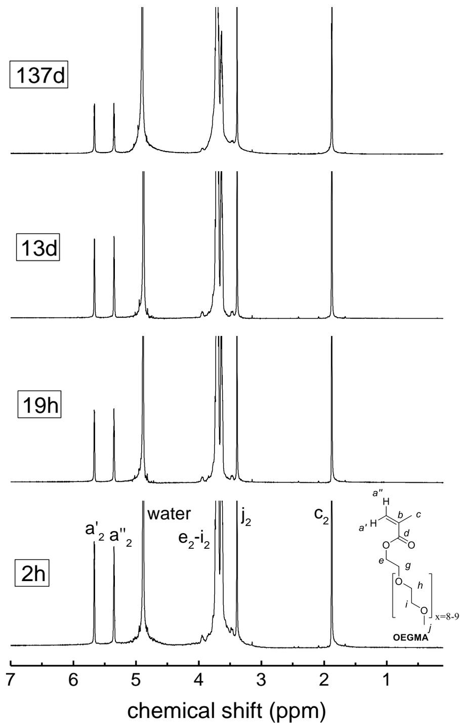
Figure S 61  $^1\text{H-NMR}$  spectrum showing the degradation of 0.1 M solution of OEGMA in sodium hydroxide in  $\text{D}_2\text{O}$  (pH = 14) at room temperature over time.
