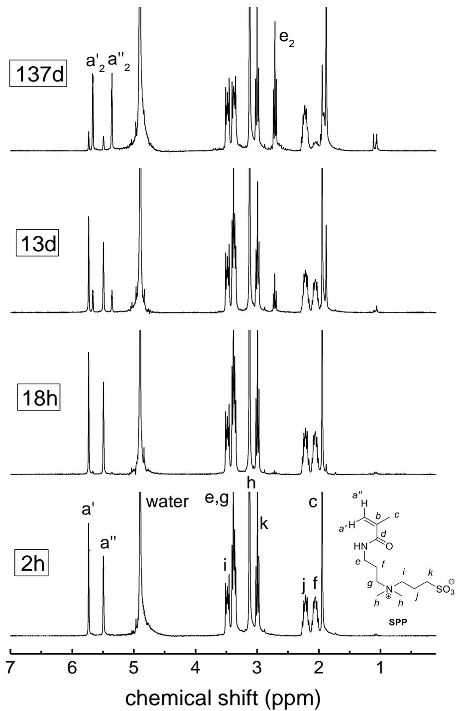
Figure S 63  $^1\text{H-NMR}$  spectrum showing the degradation of 0.1 M solution of **SPP** in sodium hydroxide in  $\text{D}_2\text{O}$  (pH = 14) at room temperature over time.
