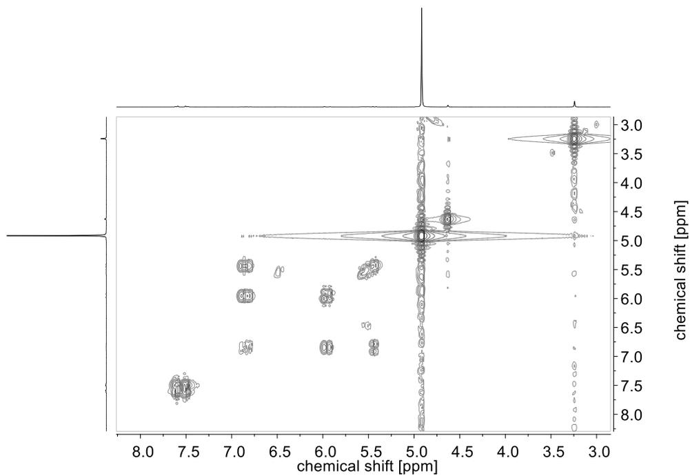
Figure S 76  $^1\text{H}$ - $^1\text{H}$ -COSY NMR spectra of 0.1 M solution of **M-5** sodium hydroxide in  $\text{D}_2\text{O}$  (pH = 14), after 124 days.
