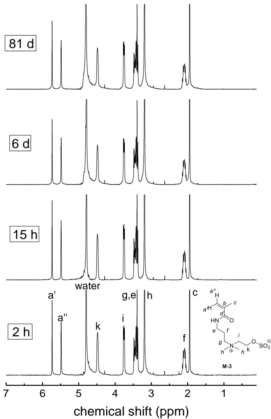
Figure S 55  $^1\text{H-NMR}$  spectrum showing the degradation of 0.1 M solution of **M-3** in carbonate buffer in  $\text{D}_2\text{O}$  (pH = 10) at room temperature over time.
