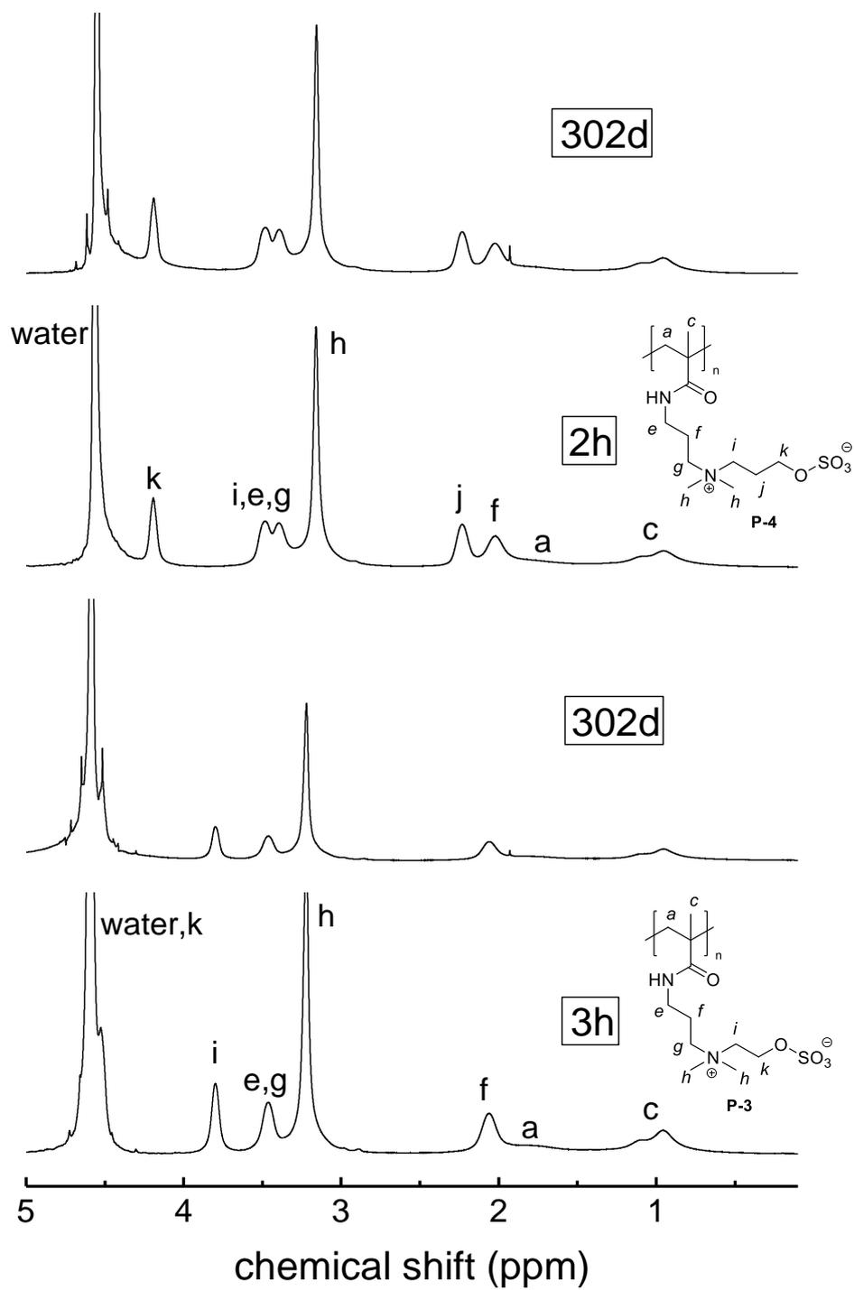
Figure S 93  $^1\text{H-NMR}$  spectrum showing the degradation of **P-3** and **P-4** in carbonate buffer in  $\text{D}_2\text{O}$  saturated with sodium chloride (pH = 10) at room temperature over time.
