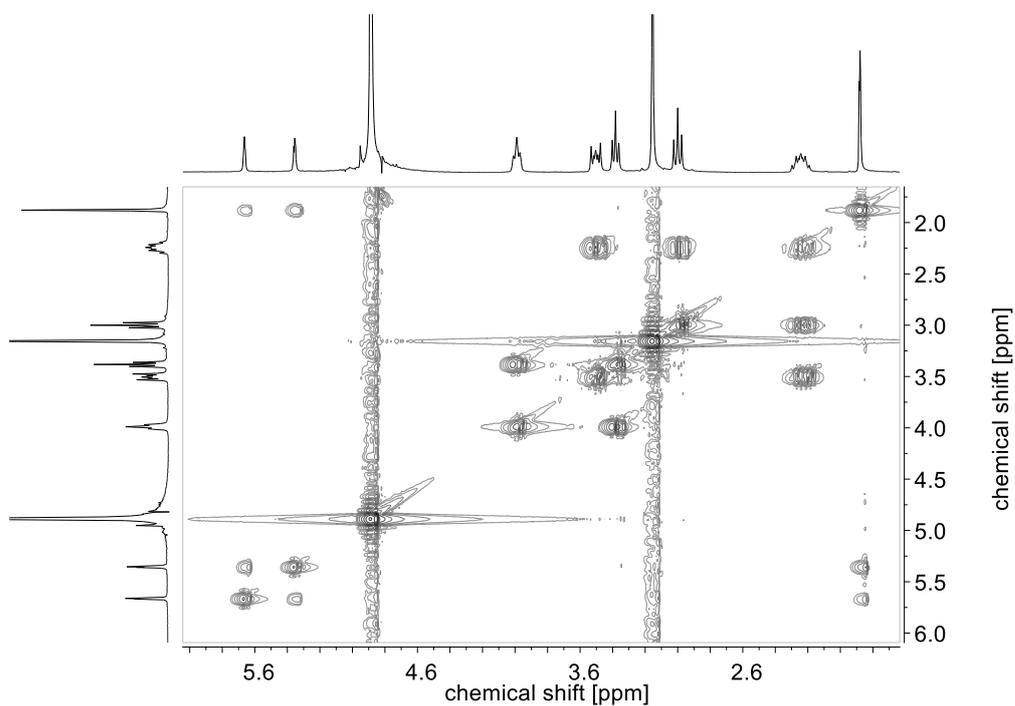
Figure S 70  $^1\text{H}$ - $^1\text{H}$ -COSY NMR spectra of 0.1 M solution of **SPE** sodium hydroxide in  $\text{D}_2\text{O}$  (pH = 14), after 124 days.
