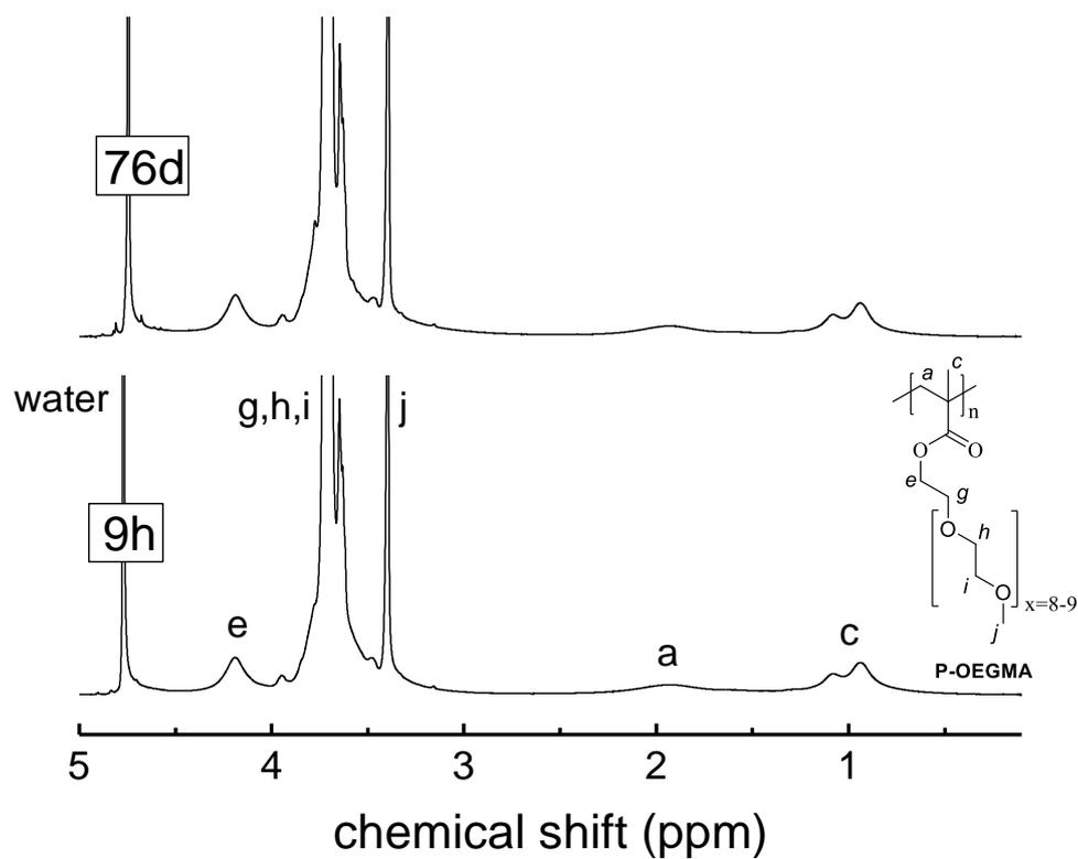
Figure S 78  $^1\text{H-NMR}$  spectrum showing the degradation of **P-OEGMA** in phosphate buffered saline (PBS) in  $\text{D}_2\text{O}$  (pH = 7.4) at room temperature over time.
