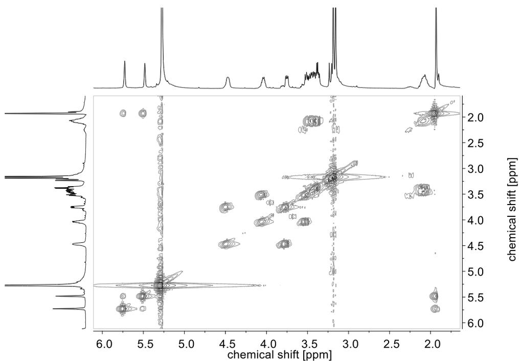
Figure S 45  $^1\text{H}$ - $^1\text{H}$ -COSY NMR spectra of 0.1 M solution of **M-3** in hydrochloric acid in  $\text{D}_2\text{O}$ , after 291 days.
