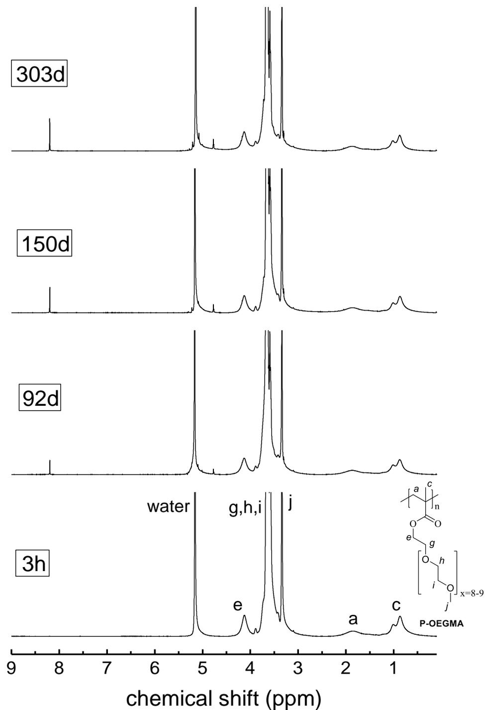
Figure S 83  $^1\text{H-NMR}$  spectrum showing the degradation of **P-OEGMA** in 1 M hydrochloric acid in  $\text{D}_2\text{O}$  (pH = 0) at room temperature over time.
