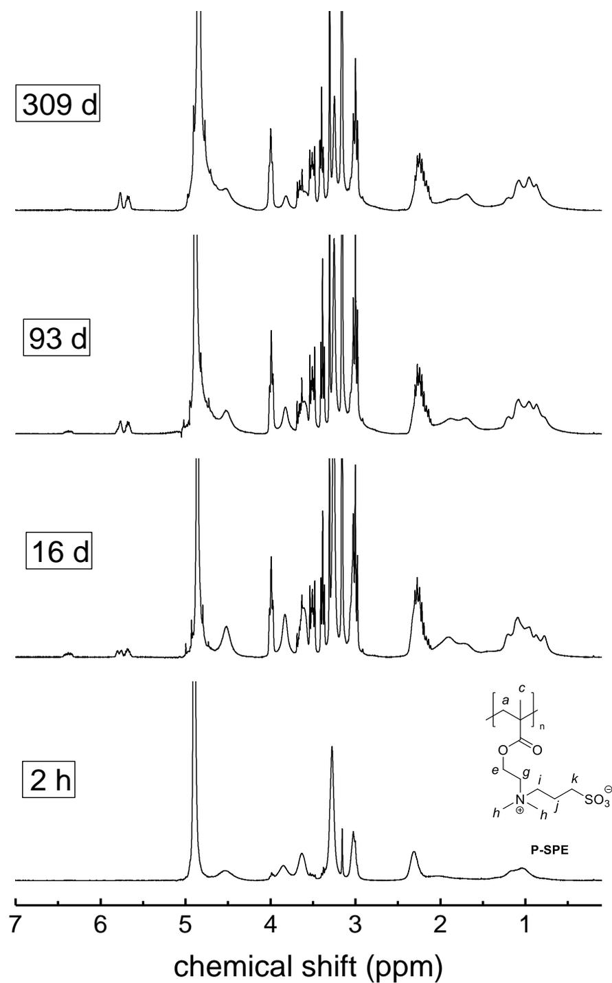
Figure S 96  $^1\text{H}$ -NMR spectrum showing the degradation of **P-SPE** in sodium hydroxide in  $\text{D}_2\text{O}$  (pH = 14) at room temperature over time.
