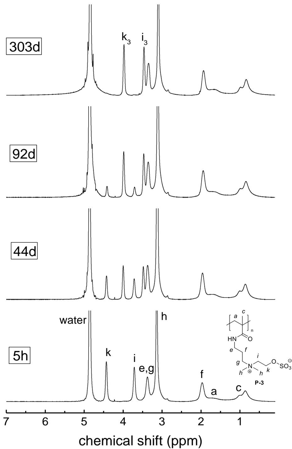
Figure S 88  $^1\text{H-NMR}$  spectrum showing the degradation of **P-3** in 1 M hydrochloric acid in  $\text{D}_2\text{O}$  (pH = 0) saturated with sodium chloride at room temperature over time.
