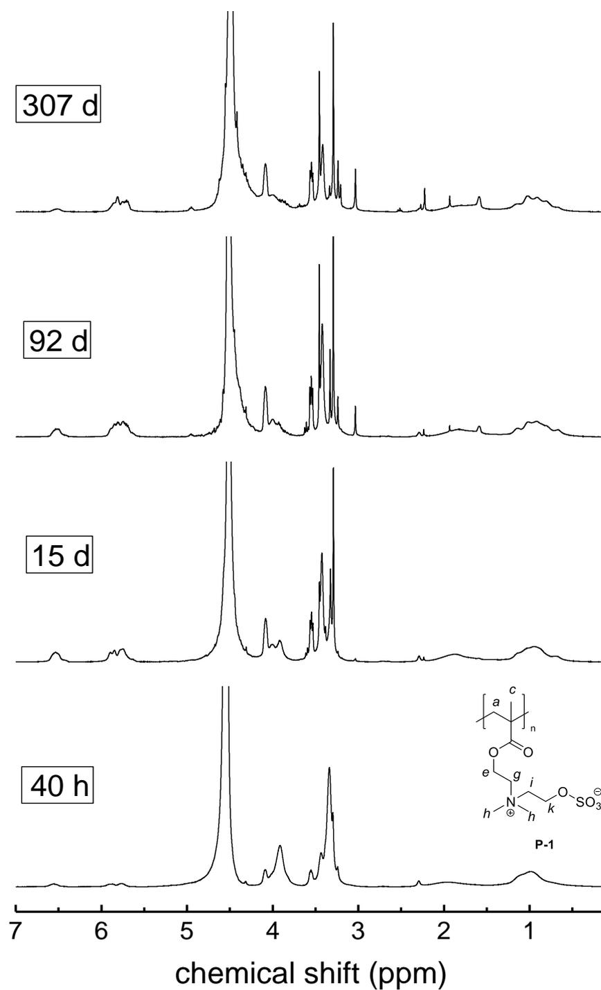
Figure S 98  $^1\text{H-NMR}$  spectrum showing the degradation of **P-1** in sodium hydroxide in  $\text{D}_2\text{O}$  saturated with sodium chloride ( $\text{pH} = 14$ ) at room temperature over time.
