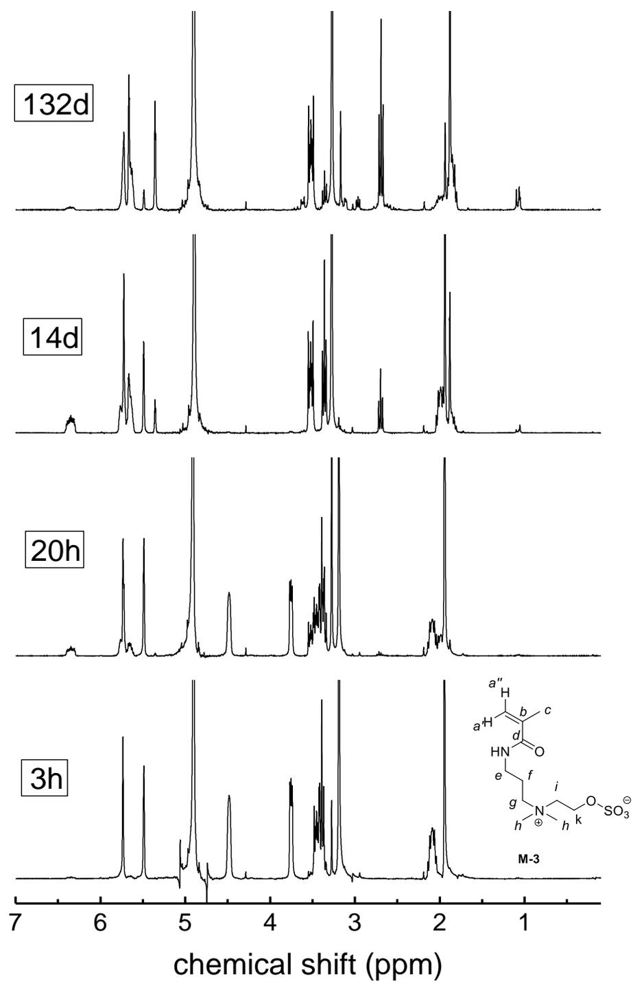
Figure S 66  $^1\text{H-NMR}$  spectrum showing the degradation of 0.1 M solution of **M-3** in sodium hydroxid in  $\text{D}_2\text{O}$  ( $\text{pH} = 14$ ) at room temperature over time.
