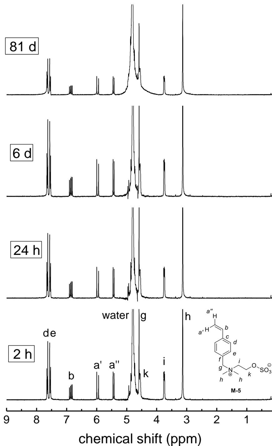
Figure S 57  $^1\text{H-NMR}$  spectrum showing the degradation of 0.1 M solution of **M-5** in carbonate buffer in  $\text{D}_2\text{O}$  (pH = 10) at room temperature over time.
