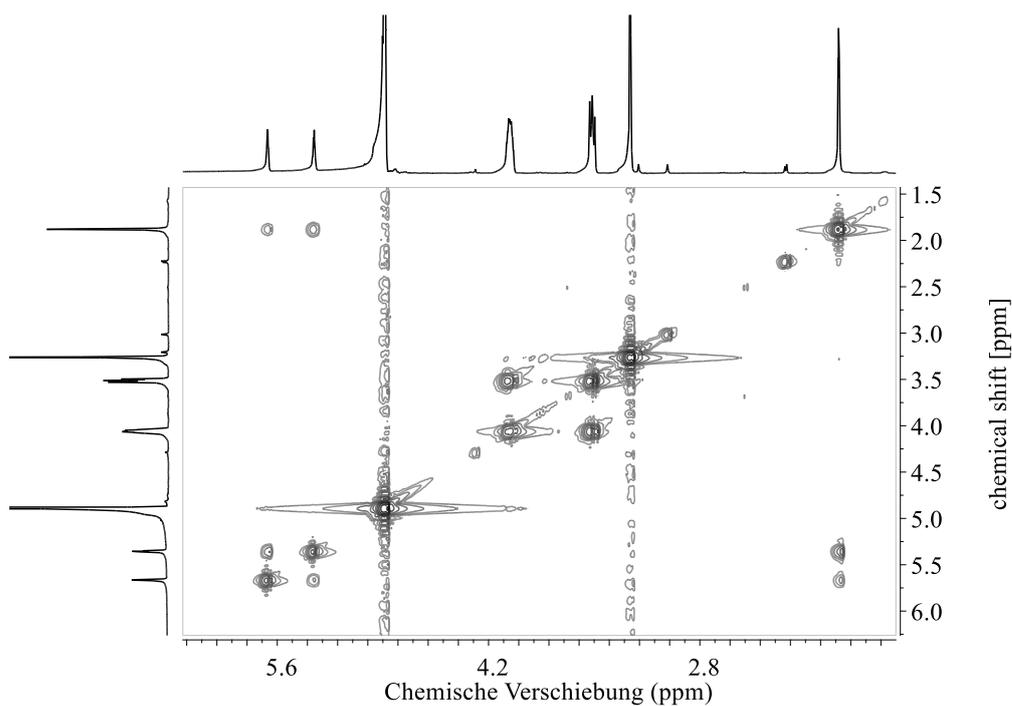
Figure S 72  $^1\text{H}$ - $^1\text{H}$ -COSY NMR spectra of 0.1 M solution of **M-1** sodium hydroxide in  $\text{D}_2\text{O}$  (pH = 14), after 124 days.
