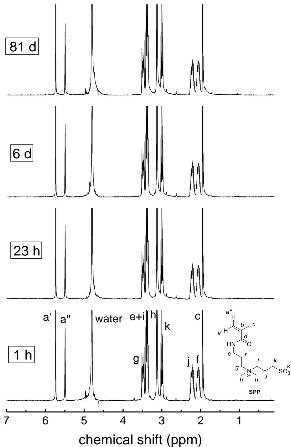
Figure S 52 <sup>1</sup>H-NMR spectrum showing the degradation of 0.1 M solution of **SPP** in carbonate buffer in D<sub>2</sub>O (pH = 10) at room temperature over time.
