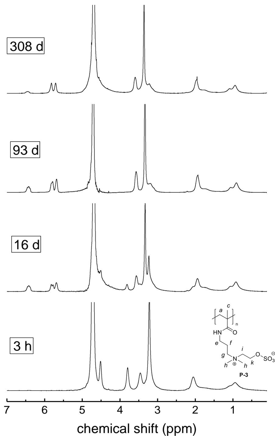
Figure S 100  $^1\text{H-NMR}$  spectrum showing the degradation of **P-3** in sodium hydroxide in  $\text{D}_2\text{O}$  saturated with sodium chloride ( $\text{pH} = 14$ ) at room temperature over time.
