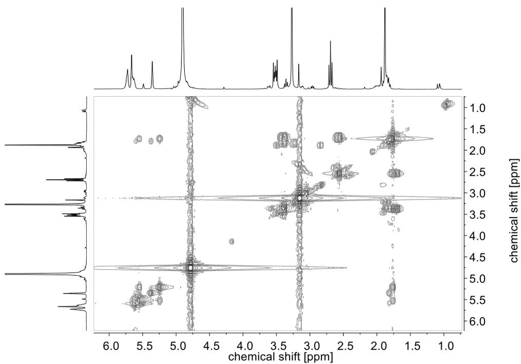
Figure S 74  $^1\text{H}$ - $^1\text{H}$ -COSY NMR spectra of 0.1 M solution of **M-3** sodium hydroxide in  $\text{D}_2\text{O}$  (pH = 14), after 124 days.
