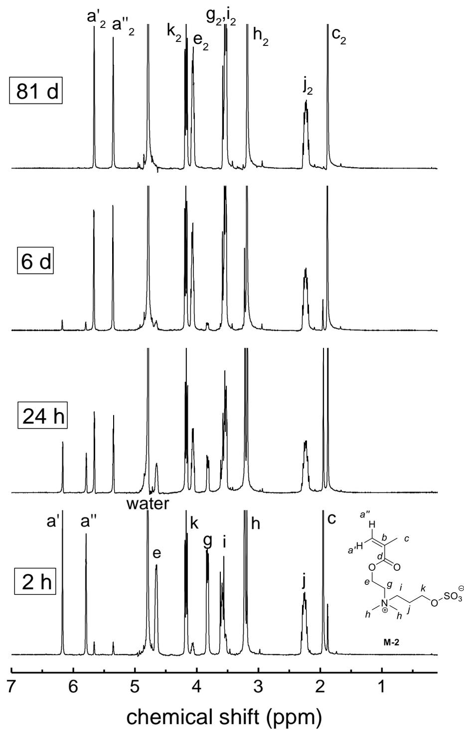
Figure S 54  $^1\text{H-NMR}$  spectrum showing the degradation of 0.1 M solution of **M-2** in carbonate buffer in  $\text{D}_2\text{O}$  (pH = 10) at room temperature over time.
