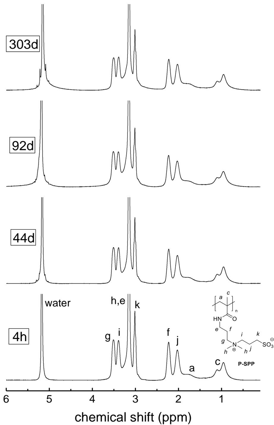
Figure S 85  $^1\text{H}$ -NMR spectrum showing the degradation of **P-SPP** in 1 M hydrochloric acid in  $\text{D}_2\text{O}$  (pH = 0) at room temperature over time.
