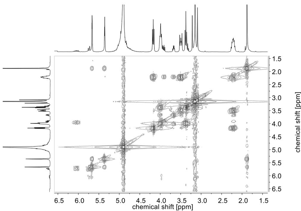
Figure S 73  $^1\text{H}$ - $^1\text{H}$ -COSY NMR spectra of 0.1 M solution of **M-2** sodium hydroxide in  $\text{D}_2\text{O}$  (pH = 14), after 124 days.
