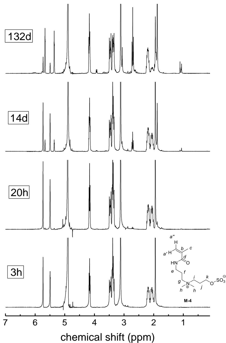
Figure S 67  $^1\text{H-NMR}$  spectrum showing the degradation of 0.1 M solution of **M-4** in sodium hydroxid in  $\text{D}_2\text{O}$  ( $\text{pH} = 14$ ) at room temperature over time.
