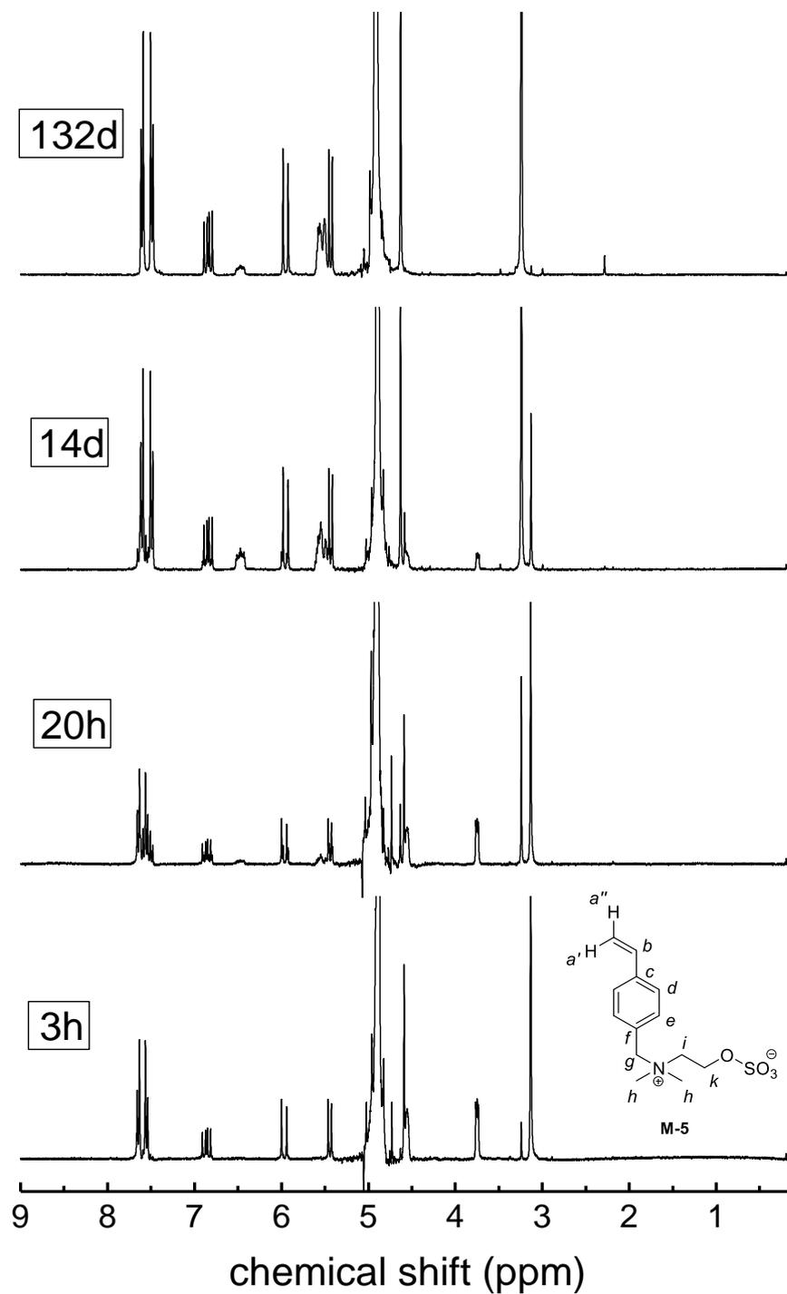
Figure S 68 <sup>1</sup>H-NMR spectrum showing the degradation of 0.1 M solution of **M-5** in sodium hydroxid in D<sub>2</sub>O (pH = 14) at room temperature over time.
