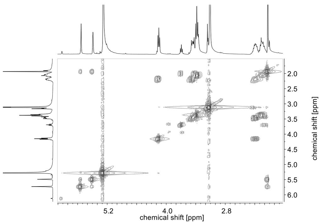
Figure S 46  $^1\text{H}$ - $^1\text{H}$ -COSY NMR spectra of 0.1 M solution of **M-4** in hydrochloric acid in  $\text{D}_2\text{O}$ , after 291 days.
