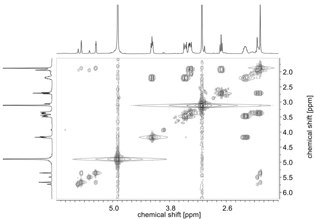
Figure S 75  $^1\text{H}$ - $^1\text{H}$ -COSY NMR spectra of 0.1 M solution of **M-4** sodium hydroxide in  $\text{D}_2\text{O}$  (pH = 14), after 124 days.
