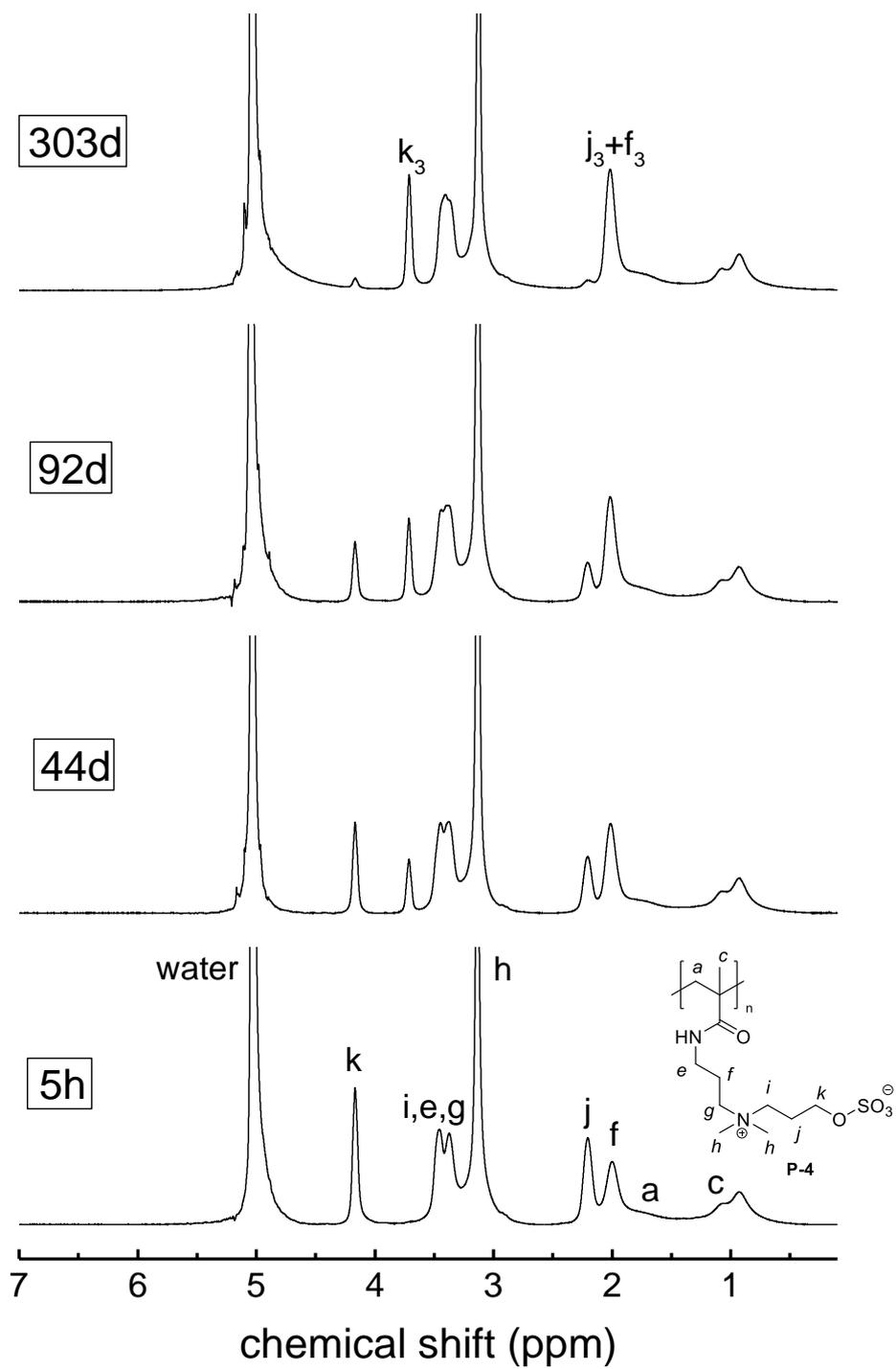
Figure S 89  $^1\text{H}$ -NMR spectrum showing the degradation of **P-4** in 1 M hydrochloric acid in  $\text{D}_2\text{O}$  (pH = 0) saturated with sodium chloride at room temperature over time.
