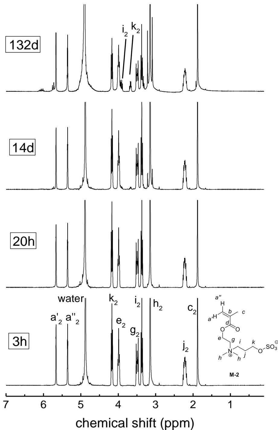
Figure S 65  $^1\text{H-NMR}$  spectrum showing the degradation of 0.1 M solution of **M-2** in sodium hydroxide in  $\text{D}_2\text{O}$  ( $\text{pH} = 14$ ) at room temperature over time.
