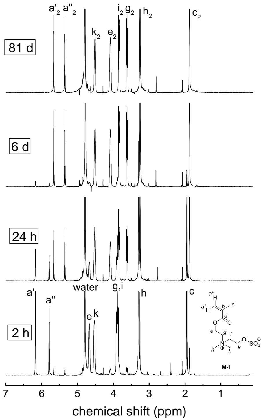
Figure S 53 <sup>1</sup>H-NMR spectrum showing the degradation of 0.1 M solution of **M-1** in carbonate buffer in D<sub>2</sub>O (pH = 10) at room temperature over time.
