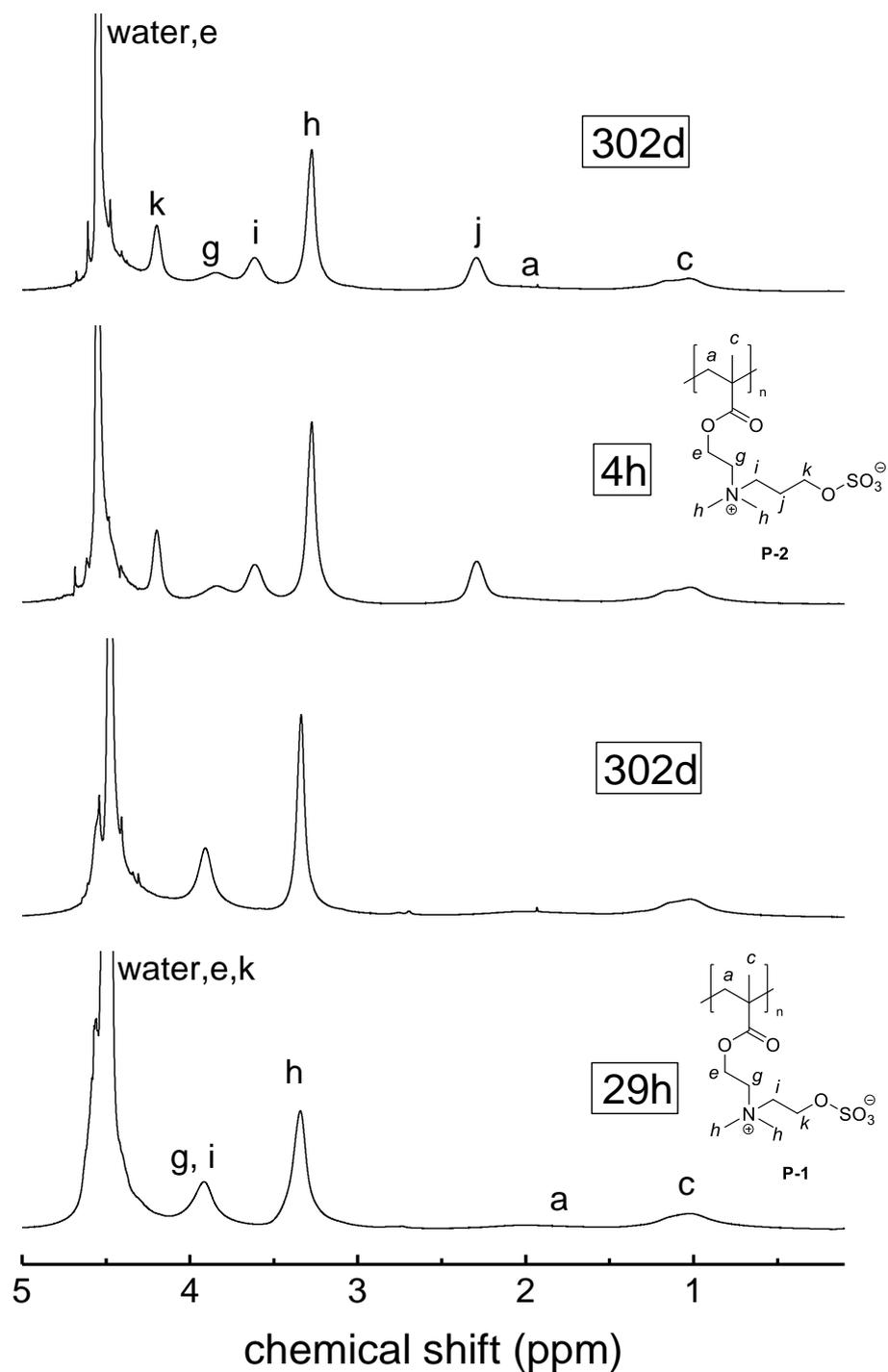
Figure S 92  $^1\text{H-NMR}$  spectrum showing the degradation of **P-1** and **P-2** in carbonate buffer in  $\text{D}_2\text{O}$  saturated with sodium chloride (pH = 10) at room temperature over time.
