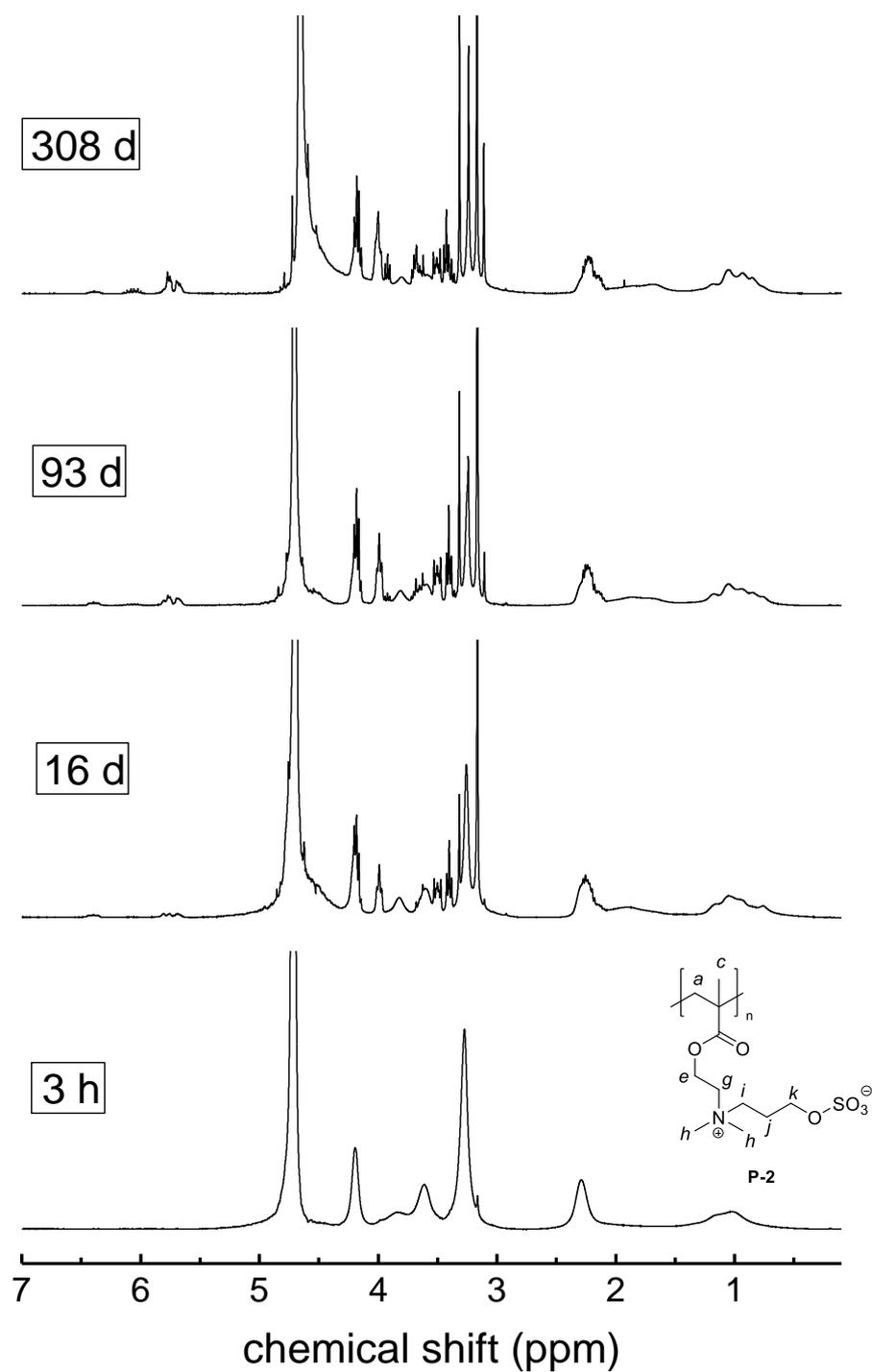
Figure S 99  $^1\text{H-NMR}$  spectrum showing the degradation of **P-2** in sodium hydroxide in  $\text{D}_2\text{O}$  saturated with sodium chloride (pH = 14) at room temperature over time.
