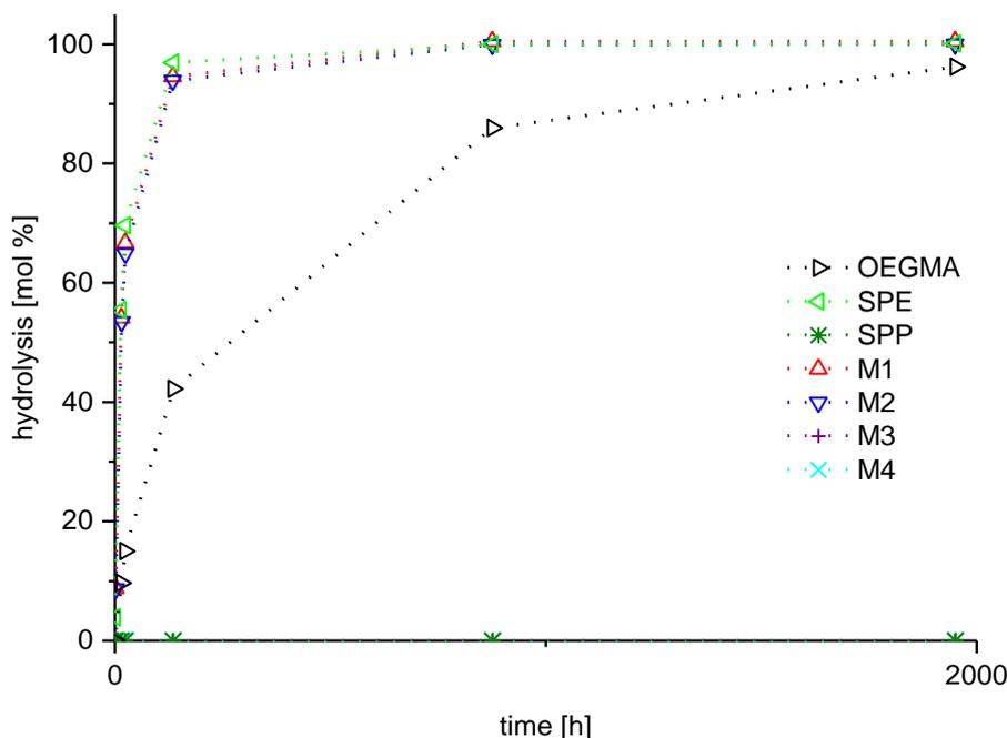
Figure S 49 Evolution of ester and amid hydrolysis of monomers in pH=10 carbonate buffer in D<sub>2</sub>O: (□) = OEGMA, (◻) = SPE, (\*) = SPP, (◻) = M-1, (◻) = M-2, (+) = M-3, (X) = M-4.
