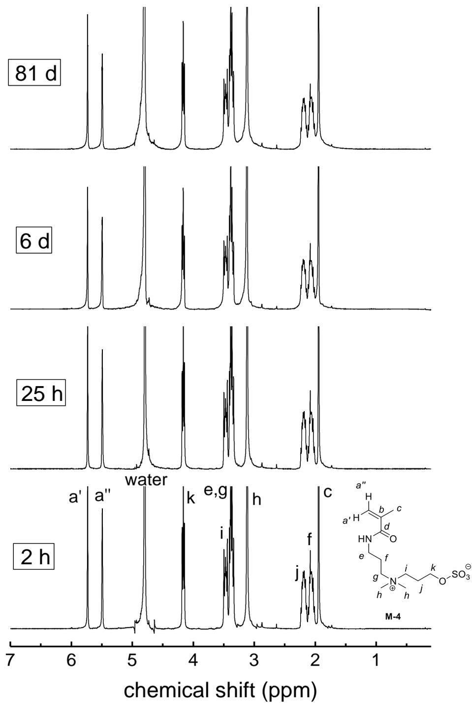
Figure S 56  $^1\text{H-NMR}$  spectrum showing the degradation of 0.1 M solution of **M-4** in carbonate buffer in  $\text{D}_2\text{O}$  (pH = 10) at room temperature over time.
