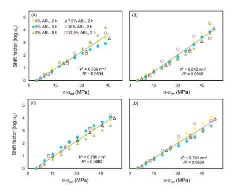
**Figure 5.** Typical Eyring equation plots of wood (**A**) and WIC<sub>SiO2</sub> with WPGs of 10% (**B**), 20% (**C**), and 30% (**D**) at a reference load of 30% ABL.
