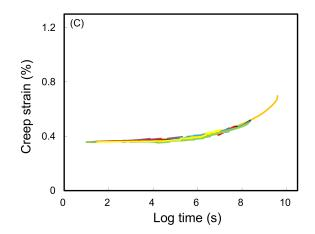
**Figure 4.** Master curves of WIC<sub>SiO2</sub> with WPGs of 10% (**A**), 20% (**B**), and 30% (**C**) using different SSM testing parameters.
