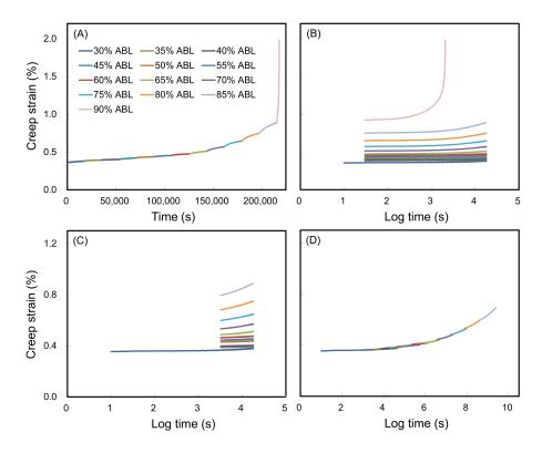
**Figure 2.** The handling of the test data of the SSM method for wood: (**A**) vertical shifting, (**B**) rescaled creep curves, (**C**) eliminating the onset time of each stress step, and (**D**) horizontal shifting.
