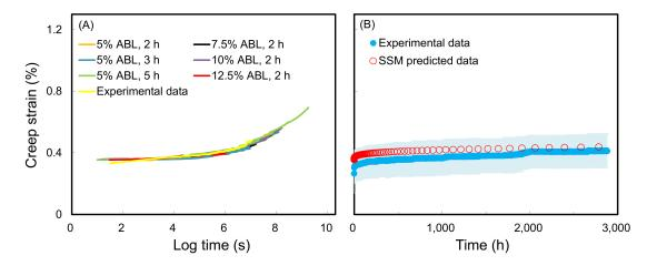
**Figure 3.** (A) Master curves of wood from different SSM testing parameters at a log time scale. (B) SSM-predicted creep curve and experimental creep data of wood at a normal time scale. Experimental data are presented as the mean (blue line)  $\pm$  SD (n = 3) (light blue ribbon).
