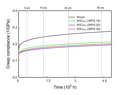
Figure 6. SSM predicted creep data of wood and WIC<sub>SiO<sub>2</sub></sub> with different WPGs.
