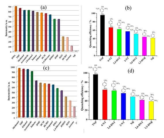
**Figure 3.** (**a**,**c**) The emission intensities of CPs **1** and **2** dispersed in different solvents ( $\lambda_{ex} = 290 \text{ nm}$ ); and (**b**,**d**) emissive response spectra of **1** and **2** for TNP in DMF solutions, respectively.
