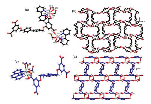
**Figure 1.** (a) The view of local coordination geometry of Cd(II) center and ligand in **1**. (b) The 2D layer in **1** as viewed slightly off the *b* axis. The hydrogen atoms have been omitted for clarity; the uncoordinated carboxyl groups pointing to the interior of pores (pink color). (c) The local coordination environment around Cd(II) in **2**. The hydrogen atoms have been omitted for clarity. (d) The 2D ladder-like layered architecture in **2**.
