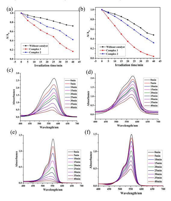
**Figure 4.** (**a**,**b**) The plot displaying photocatalytic degradation kinetics of MV and RhB in presence of of CPs **1** and **2**; and (**c**–**f**) UV–vis absorption spectra of the MV and RhB solution during the decomposition reaction under 250 W Hg lamp irradiation in the presence of CPs **1** and **2**, respectively.
