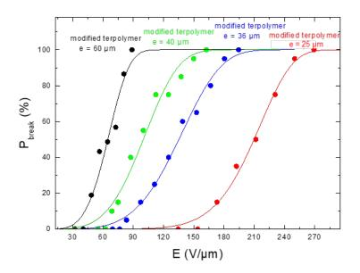
Figure 6. Breakdown probability versus electric field of modified terpolymers with different thicknesses.
