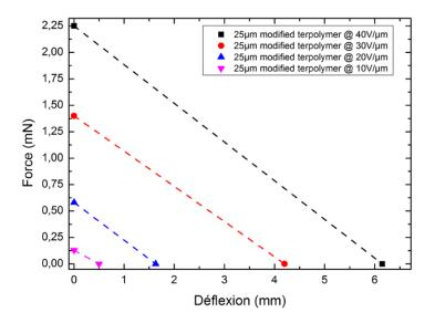
Figure 12. Actuator force versus displacement at 0.1 Hz under different electric fields.
