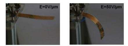
Figure 9. Photo of the unimorph under different input electric field values.
