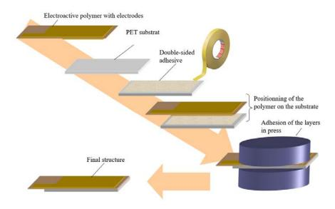
Figure 7. Fabrication process of a P(VDF-TrFR-CTFE) composite actuator.
