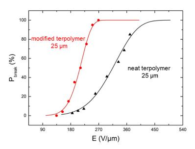
Figure 5. Breakdown probability versus electric field for different electrostrictive composites.
