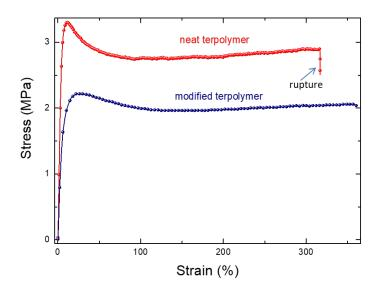
Figure 4. Longitudinal strain versus stress for different electrostrictive composites.
