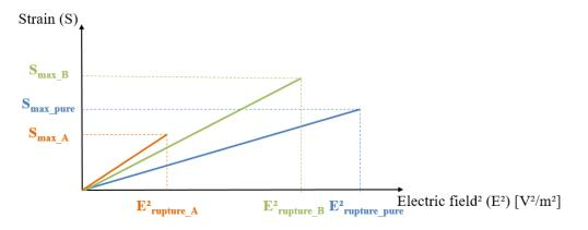
Figure 3. Strain versus electric field squares for different electrostrictive composites.
