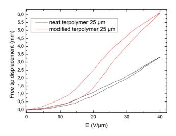
Figure 10. Free displacement versus electric field at 0.1 Hz for two terpolymer compositions.
