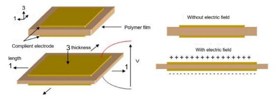
Figure 1. Principle schematic of the electrostrictive actuation.
