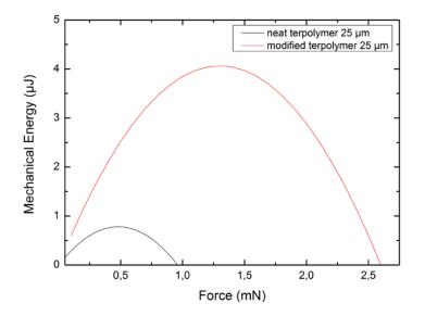
**Figure 13.** Mechanical energy density function of deflection for two compositions of terpolymer for an electric field of  $40 \text{ V}/\mu\text{m}$ .
