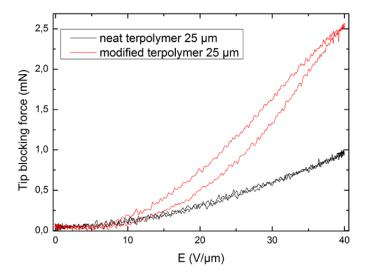
Figure 11. Blocking force versus electric field for two terpolymer compositions.
