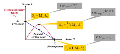
Figure 2. Pertinent parameters and figures of merit for an electroactive polymer.
