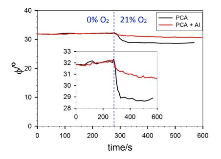
**Figure S5.** [Ru(phen)<sub>2</sub>(4-Clp)]/PCA temperature-sensitive spots in the organ-on-a-chip device: response to O<sub>2</sub> (from 0% to 21% O<sub>2</sub> in N<sub>2</sub> by volume) at 27 °C. Black line: naked T-sensitive luminescent film; red line: aluminum foil-covered T-sensitive luminescent film.
