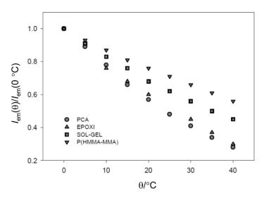
**Figure S3.** Variation with temperature of the luminescence intensity at 590 nm of the polymer monoliths doped with [Ru(phen)<sub>2</sub>(4-Clp)]<sup>2+</sup> (see Experimental section).
