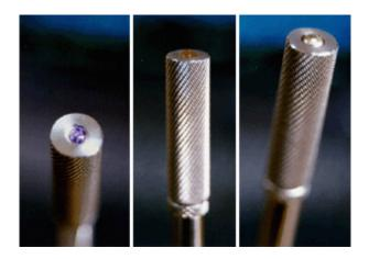
**Figure S1.** Optical fiber tip with the [Ru(phen)<sub>2</sub>(4-Clp)]<sup>2+</sup>/PCA sensitive material. Left: top view showing the blue light excitation; center: side view showing the red luminescence from the polymer terminal; right: polymer terminal covered with aluminum foil.
