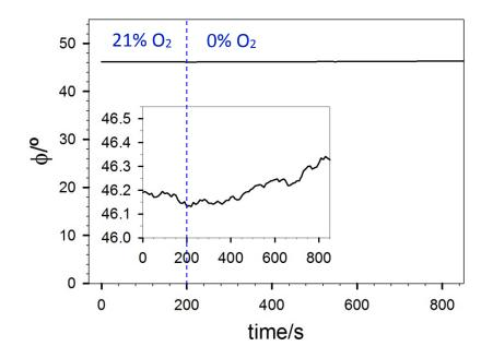
**Figure S4.** Response to O<sub>2</sub> (from 21% to 0% O<sub>2</sub> in N<sub>2</sub> by volume) of the [Ru(phen)<sub>2</sub>(4-Clp)]/PCA temperaturesensitive optical fiber tip at 25 °C. The inset shows a zoom of the y-axis of the plot.
