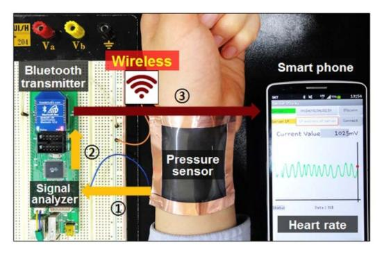
Figure 11. Photograph of wearable and wireless pressure sensor for heart rate monitoring [147].
