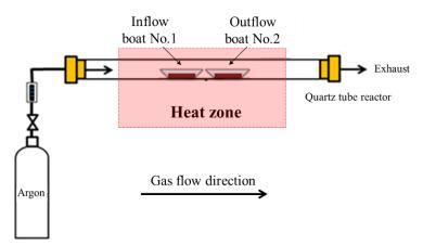
Figure S2. Schematic of the furnace system.
