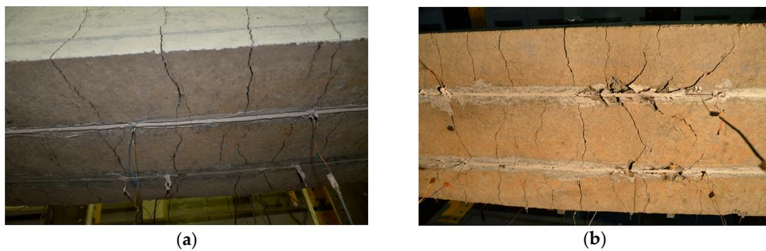
Figure 8. Cracking pattern on the bottom surface of beams of series B: (a) NSM12B; and (b) NSM12B-L.
