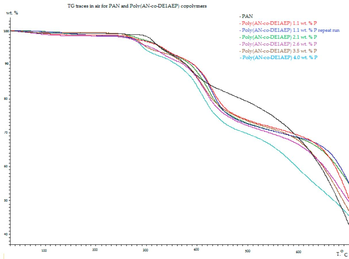
Figure S3. TG traces obtained under air for PAN and the copolymers poly(AN-co-DE1AEP) containing different amounts of phosphorus.
