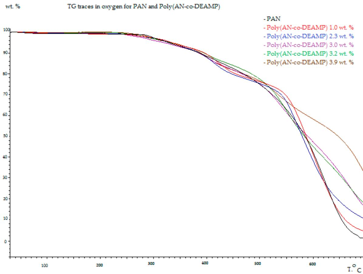
Figure S2. TG traces obtained under oxygen for PAN and the copolymers poly(AN-co-DEAMP) containing different amounts of phosphorus.
