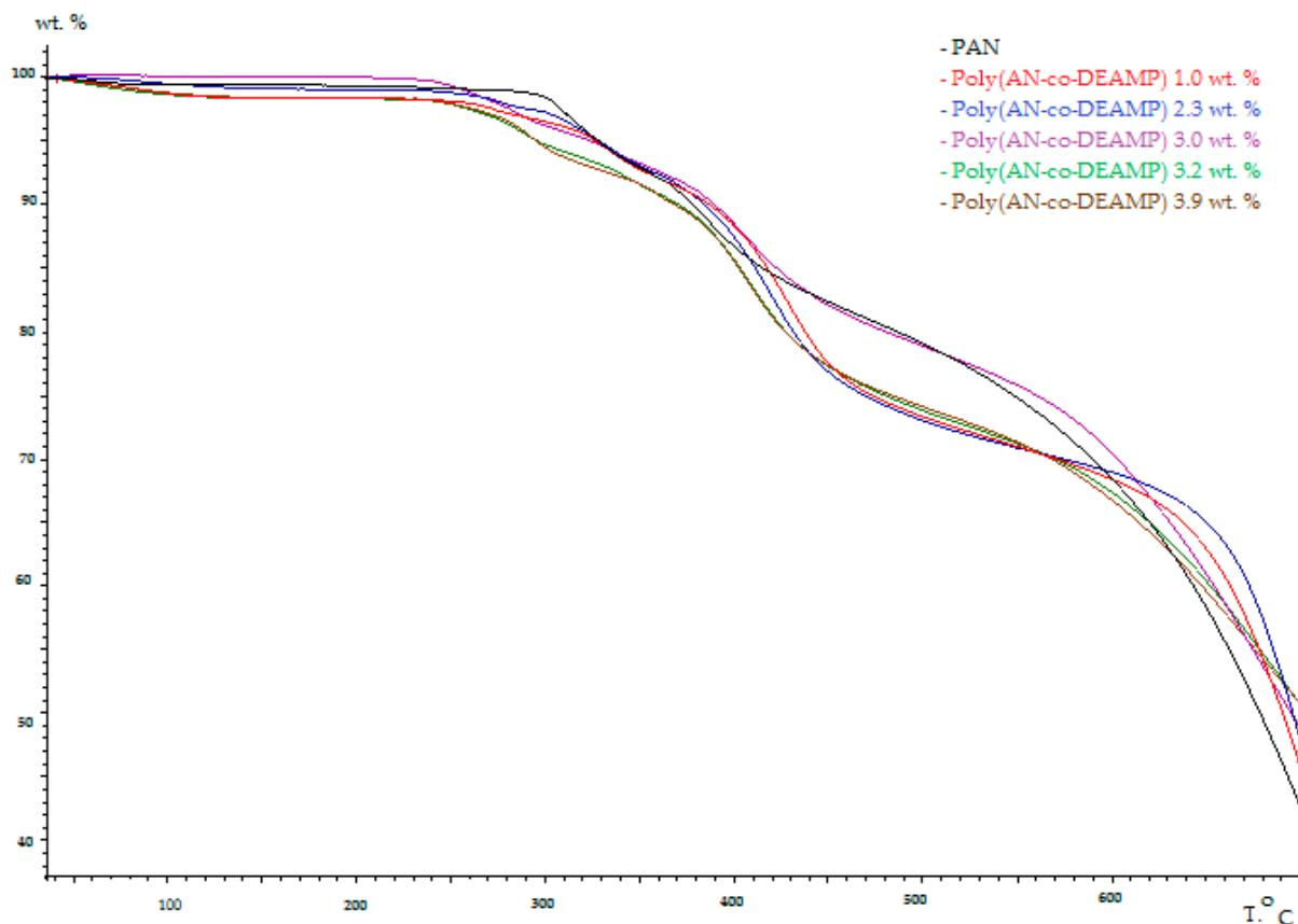
Figure S1. TG traces obtained under air for PAN and the copolymers poly(AN-co-DEAMP) containing different amounts of phosphorus.
