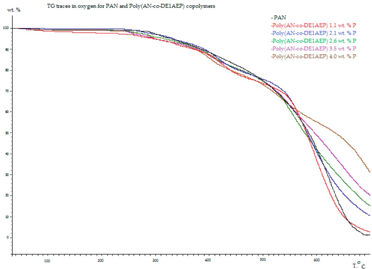
Figure S4. TG traces obtained under oxygen for PAN and the copolymers poly(AN-co-DE1AEP) containing different amounts of phosphorus.
