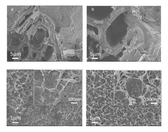
**Figure 5.** SEM images of original biocomposites (MWPC0) (**a**,**c**); magnetic biocomposites (MWPC20) at different magnifications (**b**,**d**).
