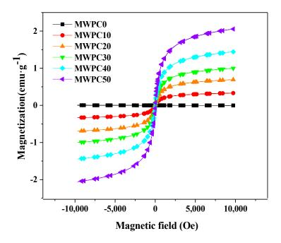
Figure 7. Magnetic hysteresis curves of the magnetic biocomposites.
