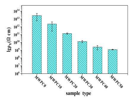
Figure 8. Volume resistivity of biocomposites.
