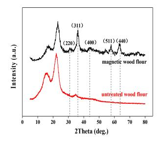
Figure 2. X-ray diffraction (XRD) patterns of the pure flour and the magnetic wood flour.
