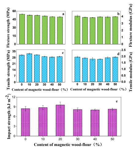
**Figure 10.** Mechanical properties of the magnetic biocomposites. (**a**) flexural strength; (**b**) flexural modulus; (**c**) tensile strength; (**d**) tensile modulus; (**e**) impact strength.
