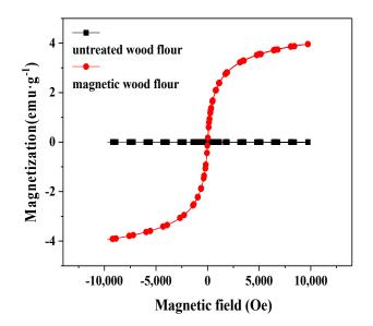
Figure 4. Magnetic hysteresis curves of the pure wood flour and the magnetic wood flour.
