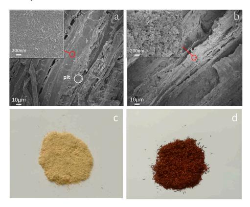
**Figure 1.** SEM images of untreated wood flour (**a**); magnetic wood flour (**b**); and the photos of untreated wood flour (**c**); magnetic wood flour (**d**).
