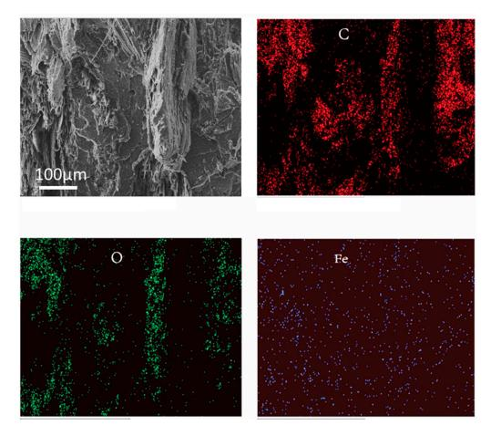
Figure 6. Energy dispersive spectroscopy (EDS) spectrum of the magnetic biocomposites (MWPC40).
