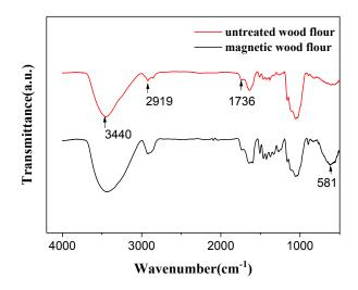
Figure 3. FTIR curves of the pure wood flour and the magnetic wood flour.
