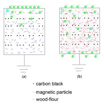
**Figure 9.** Assumed model of the synergistic effect of carbon black and magnetic lignocellulosic particles on electrical conductivity: (**a**) original biocomposites; (**b**) magnetic biocomposites.
