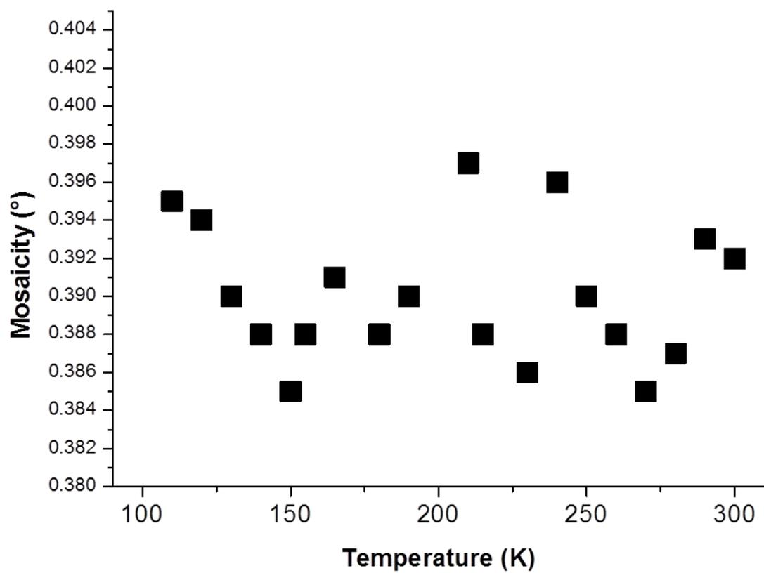
**Figure S5.** Mosaicity of the crystal test as a function of temperature, all scan parameters being strictly equal for all data collections. The influence of the temperature appears quite weak for that sample.
